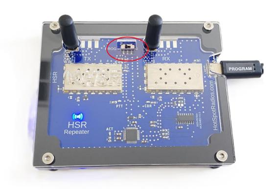
Now run the radio program again for programming the rx radio module.
