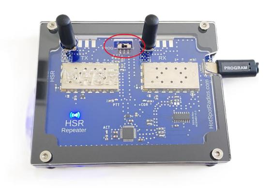
Note: You will need a minimum of 5 MHz of frequency separation between the RX radio module and the TX Radio module frequencies.
