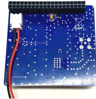
Thread the USB data cable (red and black wires) through the hole on the Pi 3B board next to the GPIO connector.
