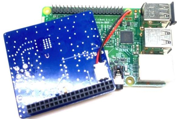
Measure and cut off excess leads on the black and red wires to solder to the USB data pads on the raspberry pi board as shown in the picture.
