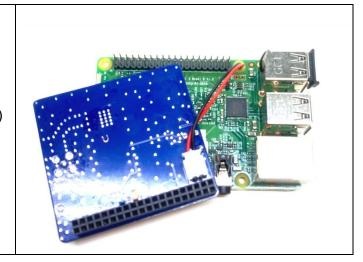
Measure and cut off excess leads on the black and red wires to solder to the USB data pads on the raspberry pi board as shown in the picture.
