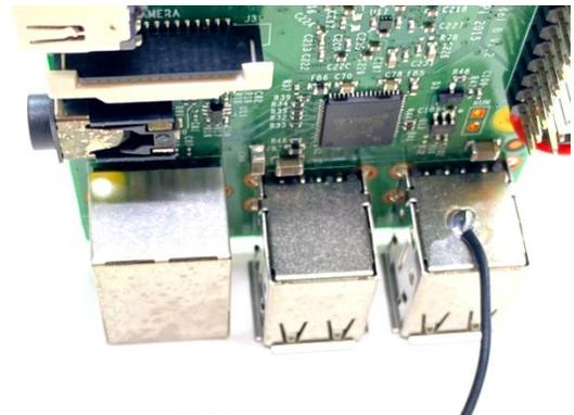
Thread the USB data cable (red and black wires) through the hole on the Pi 3B board next to the GPIO connector.
