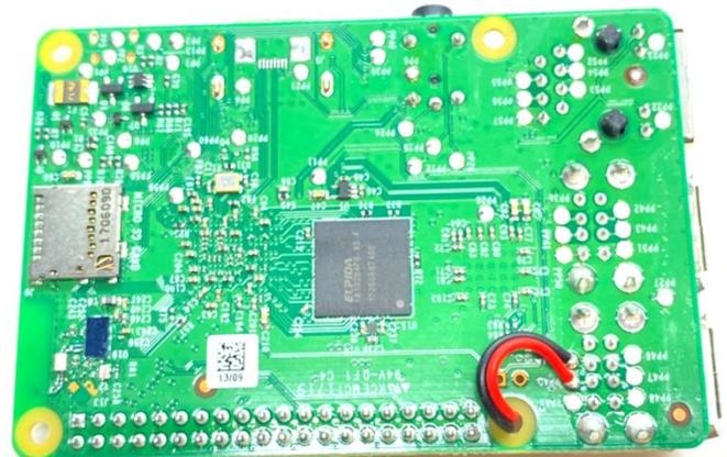
If you have purchased the custom HSR C4Labs Pi case it is now time to construct and install the Pi 3 B board into the case. Refer to the installation instructions that are included with the case for assembly. Install only the large heat sink for the main raspberry Pi CPU. Leave the small heat sink installation on the bottom of the Pi until the very end of construction.
