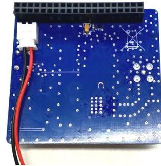
Solder one side of the provided black ground wire to of the Pi 3B USB shield housing on the raspberry Pi board as shown in the picture. This wire provides a ground to the Pi Hat HSR board.
