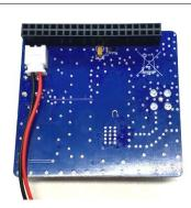
Solder one side of the provided black ground wire to of the Pi 3B USB shield housing on the raspberry Pi board as shown in the picture. This wire provides a ground to the Pi Hat HSR board.
