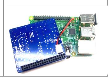
Measure and cut off excess leads on the black and red wires to solder to the USB data pads on the raspberry pi board as shown in the picture.
