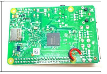
If you have purchased the custom HSR C4Labs Pi case it is now time to construct and install the Pi 3 B board into the case. Refer to the installation instructions that are included with the case for assembly. Install only the large heat sink for the main raspberry Pi CPU. Leave the small heat sink installation on the bottom of the Pi until the very end of construction.
