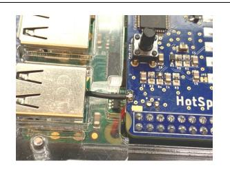
You can now refer back to C4Labs instruction sheet for installation of Items 10 and 11. Proceed with installing Items 10 and 11, the black housing level and the clear top cover with the HSR logo. Lastly Install the small heat sink on the bottom of the Pi.
