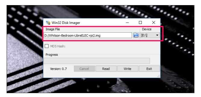
When you've got it set up, click the "Write" button. This overwrites the SD card's data with data from the cloned image.
