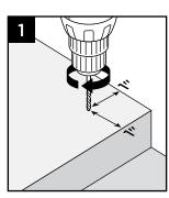
For best results using an 18V or higher cordless drill and the included HEXSTIX<sup>®</sup> depth setter, install fasteners at a 90° angle (perpendicular to the board). Drive the screws into the decking until the bit releases from the screw.
