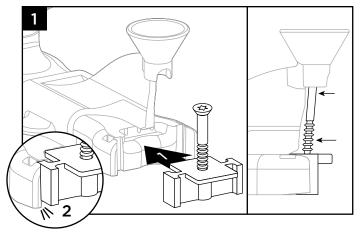
1. Place Hideaway hidden fastener into one-step tool. There will be a slight click when fastener is engaged properly. Screw will also be slightly at an angle when engaged in one-step tool properly.
