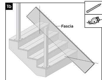
1b. Another option is cutting fascia plumb to the rim joist at the top and flush at the bottom of the stairs as shown.
