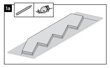
1a. Using a stair stringer as a template, lay this on the fascia and trace out pattern for stair stringer, ensuring you also factor in stair tread/deck board thickness and riser thickness before cutting. This option is shown above. Proceed to step 3.
