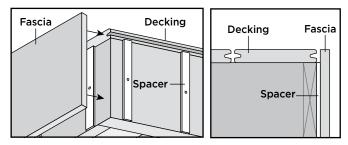
Install 3/16" to 1/4" thick x minimum 1" wide exterior grade spacers (these should be cut the same length as the rim joist), and spaced 9" on center. Install fascia screws as stated below at spacer locations (ensure that spacer screw does not interfere with fascia screw).
