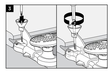
3. Using bit included with one-step tool, install screw as shown. Screw should be slightly countersunk into fastener when installed correctly. Continue to install fasteners on every joist. **Do Not Overdrive Screw**.
