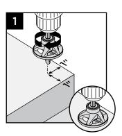
Using the HEXSTIX<sup>®</sup> depth setter in a 18v or greater drill or impact driver, install fasteners at a 90° angle (perpendicular to the board). Drive the screws into the decking until the bit releases from the screw.
