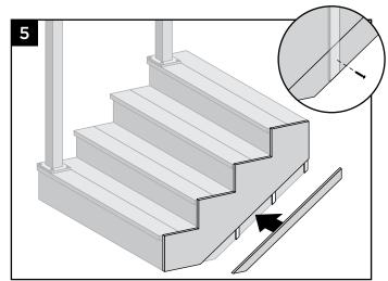
5. If the fascia is not wide enough to cover the stair stringer, a secondary piece of fascia may need to be cut accordingly and installed. Install using one recommended fascia fastener on or near the spacer.
