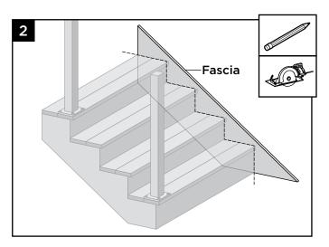
2b. Once completed place fascia in proper location and trace around stair treads and risers and then cut to fit.
