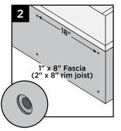
When using 2" x 10" or larger framing (1x12 fascia applications), bore 3 holes into the fascia every 18" ensuring that holes are starting and ending 1" away from the ends of the fascia as well as 1" from the bottom and top of the rim joist.
