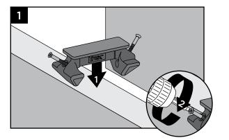
1. For butt joints, where boards meet over a single joist, install butt clip to shared joist as shown with 2 screws (supplied with clip).
