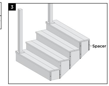
3. Spacers should be installed like that of standard decking, ensuring these are spaced 9" apart (see previous page for detailed information on all requirements for spacers).
