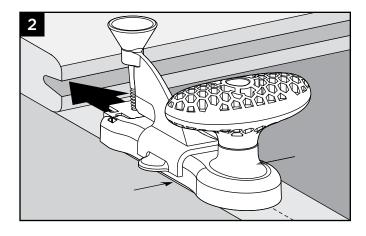
2. Center one-step tool (with fastener included) on joist and push into groove of board.
