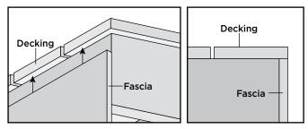
Install fascia **UNDER** decking edges/ends. This will optimize the aesthetics and performance of the installation.
