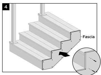
4. Install appropriate number of recommended fasteners as per pattern shown above, as overall size of fascia after being cut may be smaller than that of the standard size, thus the number of screws used every 18" may be different in different areas. Ensure screws are installed 1" from edge of stringer (do not install screws in the end of the stair tread).
