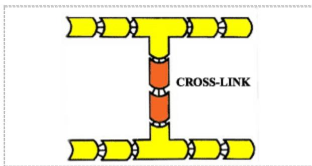
A polymer with too much cross-linking is brittle and easily shattered. However, cross-linked polymers can be made stronger with IPN's (Interpenetrating Polymer Network). Imagine weaving a strong polymer rope through the holes of the cross-linked net. This rope will add strength to the net without causing brittleness.
