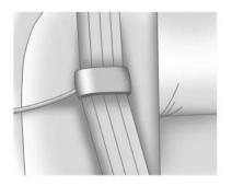
Be sure that the belt is not twisted and it lies flat. The elastic cord must be under the belt and the guide on top.
