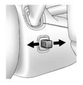
The switch used to adjust the pedals is located on the right side of the steering column, below the wiper stalk.
