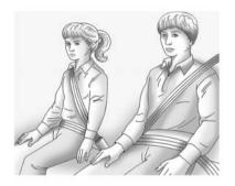
Older children who have outgrown booster seats should wear the vehicle safety belts. The manufacturer's instructions that come with the booster seat state the weight and height limitations for that booster. Use a booster seat with a lap-shoulder belt until the child passes the fit test below:
