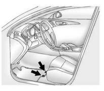
1. Pull up on the rear of the floor mat to unlock each retainer and remove.
