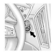
The vehicle has an electronic keyless ignition with pushbutton start.
