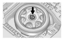
4. Remove the nut retaining the spare tire.
