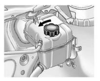
Remove the coolant surge tank pressure cap when the cooling system, including the coolant surge tank pressure cap and upper radiator hose, is no longer hot.
