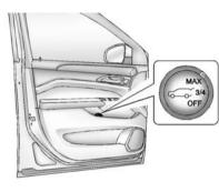
On vehicles with a power liftgate the switch is located on the driver door. The vehicle must be in P (Park) to use the power feature. The taillamps flash when the power liftgate moves.
