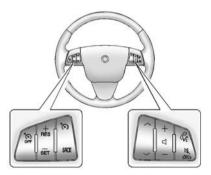
Use these controls, if equipped, to make audio adjustments at the steering wheel.
