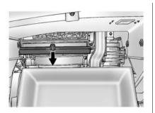
4. Release the two latches holding the service door. Lower the service door.
