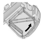
For vehicles with a u-rail system, the fence can be moved to different positions on the u-rail track to secure cargo.
