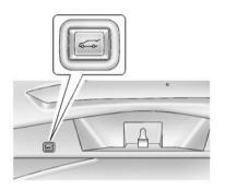
Press and release  $\iff$  on the liftgate next to the latch to close the liftgate.
