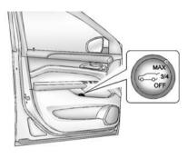
On vehicles with a power liftgate, the switch is on the driver door. The vehicle must be in P (Park) to use the power feature. The taillamps flash when the power liftgate moves.
