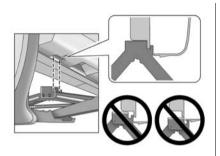
Raise the vehicle by turning the wheel wrench clockwise until the slots in the jack head fit into the metal flange located behind the triangle on the plastic moulding.
