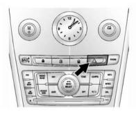
(Hazard Warning Flashers): Press this button on the instrument panel, to make the front and rear turn signal lamps flash on and off. This warns others that you are having trouble. Press again to turn the flashers off.
