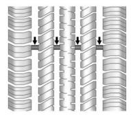
Treadwear indicators are one way to tell when it is time for new tires. Treadwear indicators appear when the tires have only 1.6 mm (1/16 in) or less of tread remaining. See *Tire Inspection on page 10-63* and *Tire Rotation on page 10-63* for more information.
