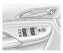
Pushing or pulling the switch part of the way will open or close the window as long as the switch is operated.
