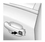
When all doors are closed and the ignition is off, the vehicle can be locked by pressing this area on the door handle. This feature will be available for several minutes after the vehicle has been turned off.
