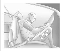
When riding in a vehicle, you travel as fast as the vehicle does. If the vehicle stops suddenly, you keep going until something stops you. It could be the windshield, the instrument panel, or the safety belts! When you wear a safety belt, you and the vehicle slow down together. There is more time to stop because you stop over a longer distance and, when worn properly, your strongest bones take the forces from the safety belts. That is why wearing safety belts makes such good sense.
