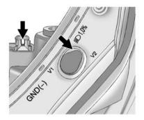
Locate the vertical headlamp adjusters, which are under the hood near each headlamp assembly.
