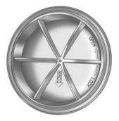
1. From the back side of the headlamp assembly, remove the top cap to replace the low-beam headlamp/DRL bulb.
