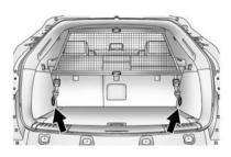
5. Mount the cargo net to the cargo tie-downs located on the lower side panels.
