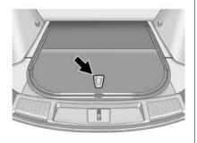
2. Press on the bottom of the handle assembly to unlatch it and lift up on the handle.
