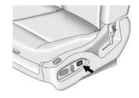
If available, press and hold the front or rear of the control to increase or decrease lumbar support. Release the control when the seatback reaches the desired level of lumbar support.
