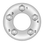
16. Tighten the wheel nuts firmly in a crisscross sequence, as shown.
