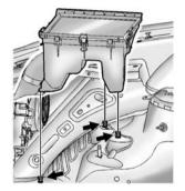
7. Lift the air cleaner/filter base to disengage from three pins.
