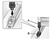
Insert the fence into the adapters and lock both latches (A) by turning to align  $\widehat{\phantom{a}}$  with the arrow on the adapter (B).
