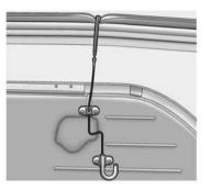
4. Store the cargo management system cover by hooking it onto the weatherstrip.
