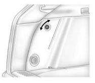
The rear compartment fuse block is located in the cargo area, on the driver side of the vehicle behind the lower trim panel. To open, turn the latch with a flat bladed tool and pull the trim panel from the edges to fold it down.
