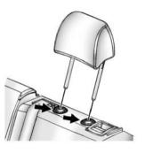
2. Press both buttons on the head restraint posts at the same time, and pull up on the head restraint.
