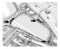
2. Unlatch three clips and lift up the underhood electrical center cover to remove.
