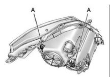
For the vehicle equipped with an up-level headlamp (HID), there will be two vertical headlamp adjusters (V1 and V2).
