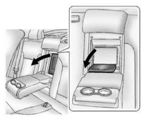
Some vehicles have a rear seat pass-through door in the center of the rear seatback. Fold down the center armrest and push down on the latch to open the door.
