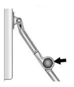
Press the red button on the prop rod to close the cover.
