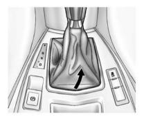
Remove the shift lever boot by pulling up on the rear of the trim plate.
