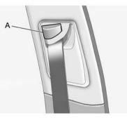
Move the height adjuster up to the desired position by pushing up on the height adjuster.
