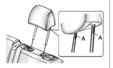
Insert the head restraint posts into the holes in the top of the seatback. The notches (A) on the posts must face the driver side of the vehicle. 2. Push the head restraint down.
