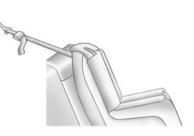
If you are using a single tether in the rear center seating position, lower the adjustable headrest down to its stowed position and route the single tether over the headrest.  Before placing a child in the child restraint, make sure it is securely held in place. To check, grasp the child restraint at the LATCH path and attempt to move it side-to-side and back-and-forth. There should be no more than 2.5 cm (1 in) of movement for proper installation.
