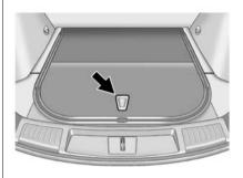
To open the cargo management system, press the handle to unlatch and then lift up.
