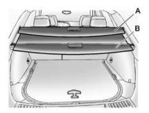
The shade can be set in two positions. It can be set in a halfway open (A) position for loading objects into the rear compartment, or the lower (B) position to conceal objects in the rear compartment.
