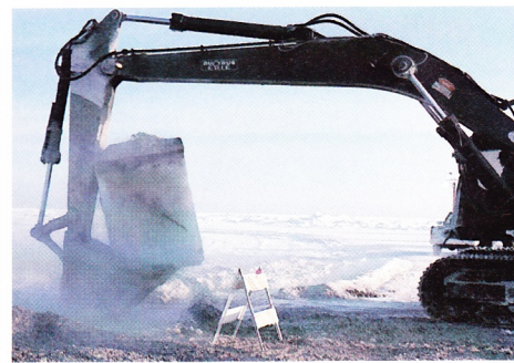
Backhoes are used to remove the individual ice blocks, some of which weigh more than 8,000 pounds, from the checkerboard.
