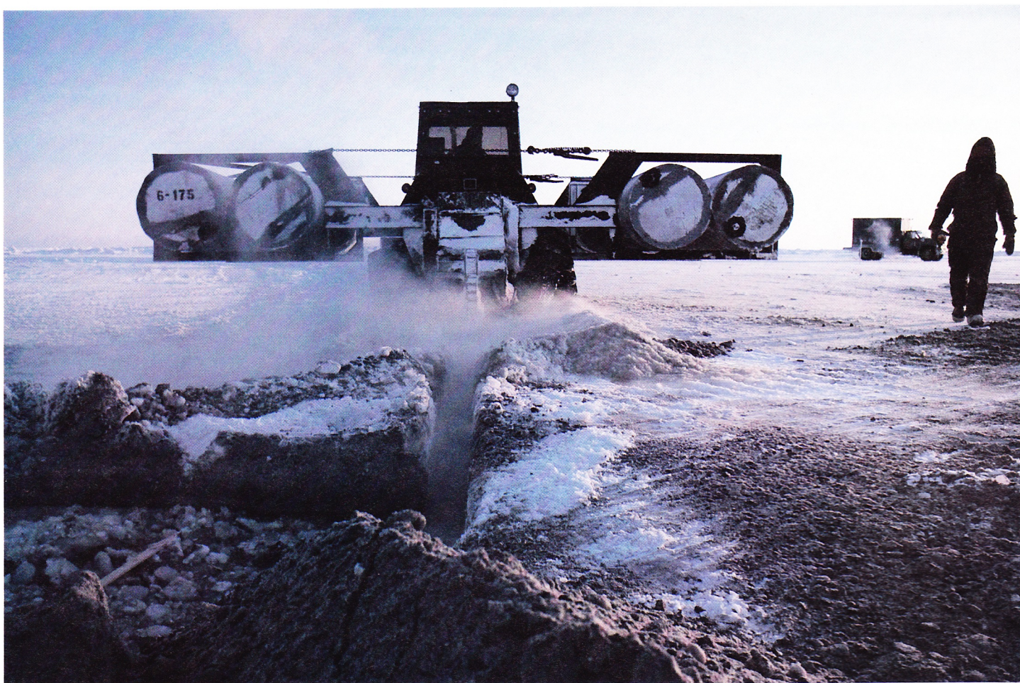
A tractor equipped with pontoons and a ditch witch slices trenches in the ice to form a giant checkerboard composed of five-foot cubes.
