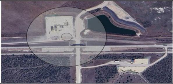
100 PPM Radius of Exposure (ROE) 677 ft untreated, 90 ft when treated
