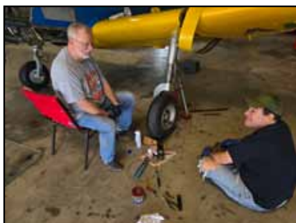
Colonels Summerall and Higginbotham ensure proper tire pressure after repacking wheel bearings on the PT-19.
