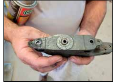
Bellcrank that had to be inspected
