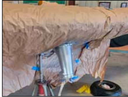
19 Strut paint job
