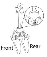
• Lower the Freedom Drive into opening of the hull near your footbraces. Use the alignment pin on each side to push the drive into the locks. The Drive lock will cover the alignment pin if done correctly.
