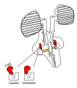
• To adjust the Freedom Drive for different height users: Squeeze the pedal adjustment bracket located on the pedal post. While squeezing bracket, move the pedal post to a more comfortable position. Remember that your legs should not fully extend as this can cause your knees to lock. Make sure the metal pin has correctly seated in the adjustment hole for each pedal post.
