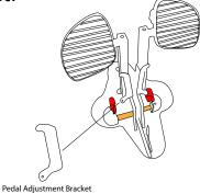
• To find the correct pedal position for the Freedom Drive, always start with the pedal posts in the 4th position when installing the drive. When you have the seat where you want it, put your feet on both pedals and the fins straight down, your knees should be comfortably bent. If your knees are over extended (straight) or too close to your chest (over stretched), try another pedal position until your knees are comfortably bent.
