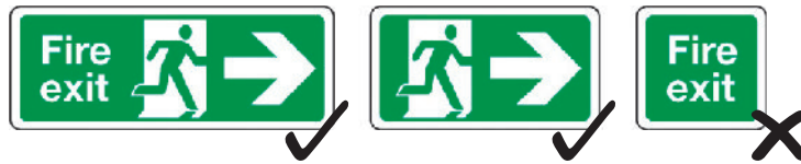
Figure 1.4 Text only safety signs do not comply.
