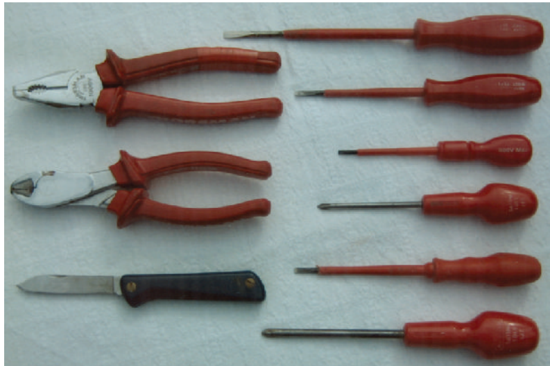
Figure 5.17 The tools used for making electrical connections.
