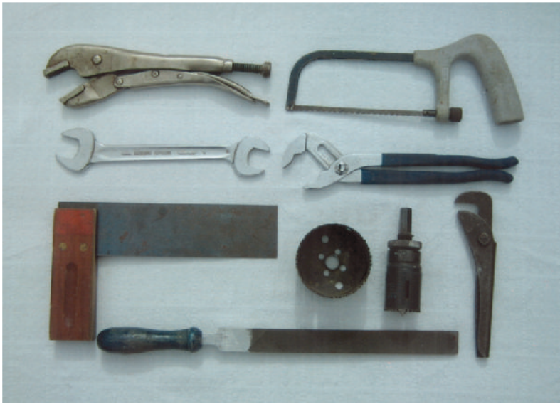
Figure 5.19 Some additional tools required by an electrician engaged in industrial installations.
