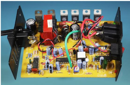
**Figure 18-1.** The interior components in a 175-watt inverter.
