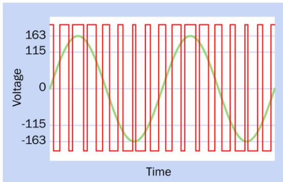
**Figure 18-5.** Pulse-width modulation adjusts the widths of pulses delivered at a high frequency. The pulse widths can be averaged to generate voltage that follows a close approximation of a sine wave.
