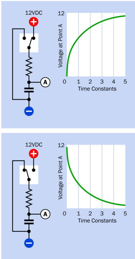
**Figure 12-3.** An RC (Resistor-Capacitor) network with a switch to control charge and discharge of a capacitor. At top, the curve gives an approximate idea of the charging behavior of the capacitor. At bottom, the curve illustrates its discharging behavior.
