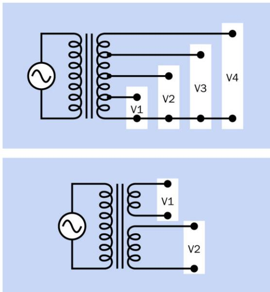
**Figure 15-6.** Multiple output voltages may be obtained from a transformer by tapping into the secondary winding (top) or using two or more separate secondary windings (bottom), in which case the outputs will be electrically isolated from each other.
