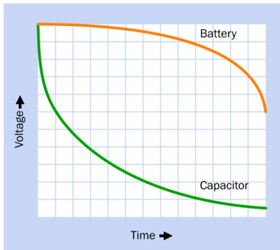
**Figure 2-5.** The voltage drop of a discharging capacitor is much steeper initially than that of a battery, making capacitors unsuitable as a battery substitute in many applications. However, the ability of a capacitor to discharge very rapidly at high amperage can sometimes be a significant advantage.
