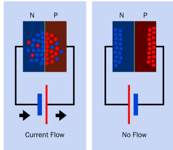
**Figure 26-4.** Inside a PN junction diode. Left: in forward-biased mode, voltage from a battery (bottom, with plates colored for clarity) forces charges in the N and P layers toward the central junction of the diode. Current begins to flow. Right: in reverse-biased mode, charges in the N and P layers are attracted away from the central junction, which becomes a depletion region, unable to pass significant current.
