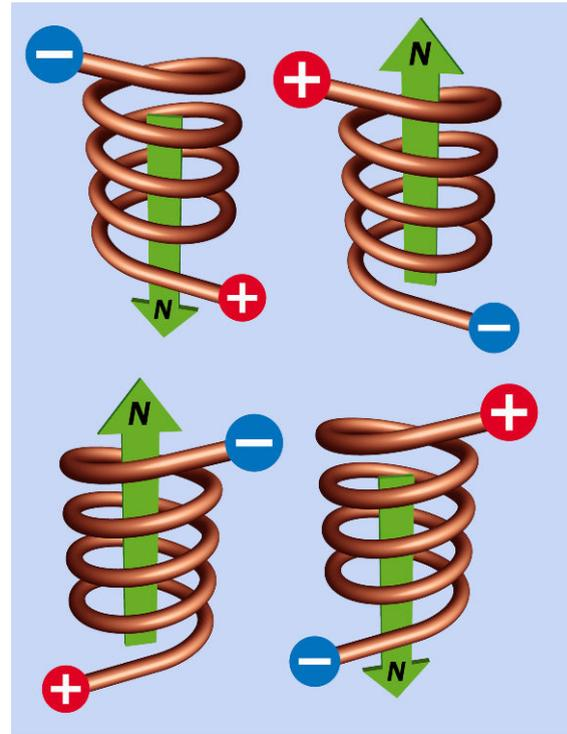
**Figure 14-6.** When DC current flows through a coil, it creates magnetic fields that will exert a force whose direction depends on the direction of the current and on whether the coil is wound clockwise or counterclockwise. The force is shown by the green arrow in each case.
