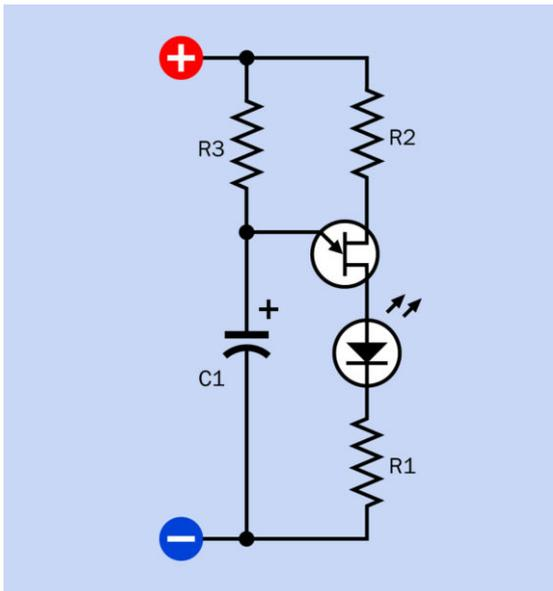
**Figure 27-8.** A basic oscillator circuit using a unijunction transistor (UJT). As the capacitor accumulates charge, the voltage on the emitter increases until it triggers the UJT, at which point the capacitor discharges through the emitter.
