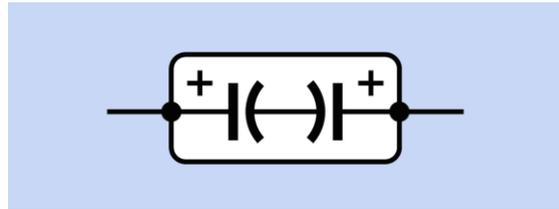
**Figure 12-12.** Schematic view of the internal configuration of a bipolar electrolytic capacitor, also known as non-polarized electrolytic capacitor. It consists of two electrolytics in series, with opposing polarities.
