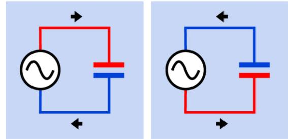
**Figure 12-4.** In the left diagram, a source of alternating current charges the upper plate of a capacitor positively and the lower plate negatively. This process entails a flow of conventional current shown by the arrows. A moment later, when the AC current flow reverses, the flow also reverses, creating the impression that the capacitor “passes” AC current.
