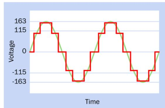
**Figure 18-4.** A secondary stream of narrower square-wave pulses can improve the fidelity of an inverter's output.
