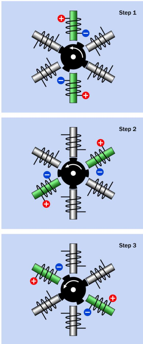
**Figure 25-2.** In a variable reluctance stepper motor, the rotor moves to minimize magnetic reluctance each time the next pair of coils is energized. At each step, the coils have been energized a moment before the rotor has had time to respond.
