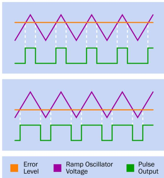
**Figure 17-2.** To achieve pulse-width modulation, an error-level voltage is established by comparing the output from the converter with a reference voltage. The error level, shown as an orange line, is then subtracted from the output from a ramp oscillator. The pulse width varies accordingly.
