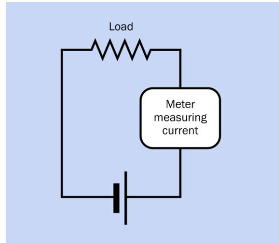
**Figure 2-11.** When measuring current using an ammeter (or a multimeter configured to measure amps), the meter must be placed in series with the battery and a load. To avoid damaging the meter, it must never be applied directly across the terminals of the battery, or in parallel with a load. Be careful to observe the polarity of the meter.
