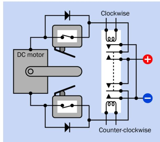
**Figure 6-20.** In this schematic, normally-closed limit switches are opened by pressure from an arm attached to a motor, thus switching off its power at each end of its permitted travel and preventing overload and burnout. A two-coil latching relay activates the motor. Rectifier diodes allow power to reach the motor to reverse its rotation when a limit switch is open.
