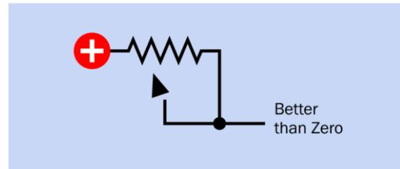
**Figure 11-12.** If the wiper of a potentiometer breaks (indicated by the loose arrow head) as a result of wear and tear, and the potentiometer is being used as a variable resistor, the voltage from it will drop to zero (top schematic) unless the wiper has been tied to one end of the track (bottom schematic).
