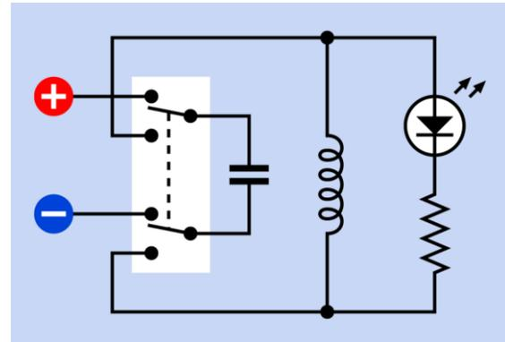
**Figure 13-5.** In this imaginary circuit, the capacitor is charged through the double-pole switch in its upper position. When the switch is turned, the capacitor forms an LC (inductance-capacitance) circuit with the coil, and resonates at a frequency determined by their values. In reality, extremely high values would be needed to obtain a visible result from the LED.
