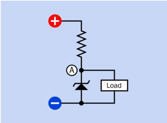
**Figure 26-19.** A simplified, basic circuit illustrating the ability of a Zener diode to compensate for variations in the power supply or load in a circuit, creating an approximately constant voltage at point A.
