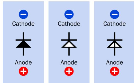
**Figure 26-1.** Commonly used schematic symbols for a generic diode. All the symbols are functionally identical. The direction of the arrow formed by the triangle indicates the direction of conventional current (from positive to negative) when the diode is forward-biased.
