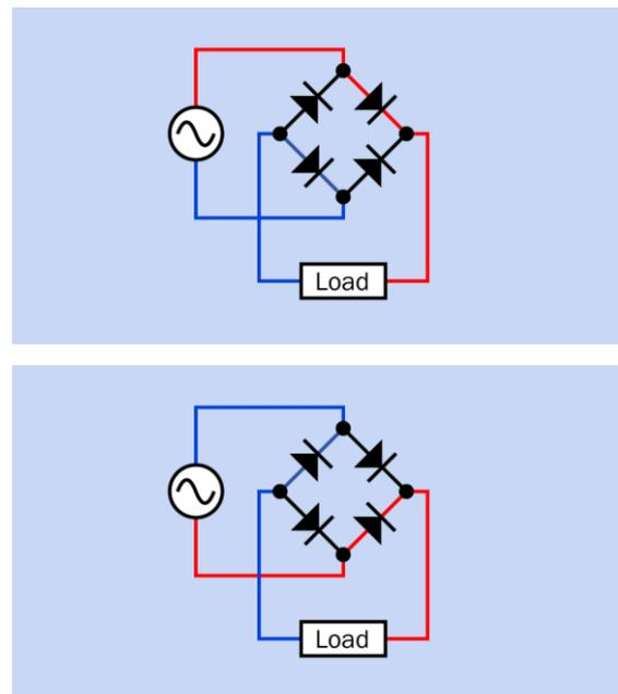
**Figure 26-9.** The basic circuit commonly used to form a bridge rectifier, with color added to indicate polarity. Wires shown in black are not passing current because diodes are blocking it. Note that the polarity at the load remains constant.
