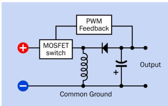
**Figure 17-5.** Basic topology of a flyback-type DC-DC converter.
