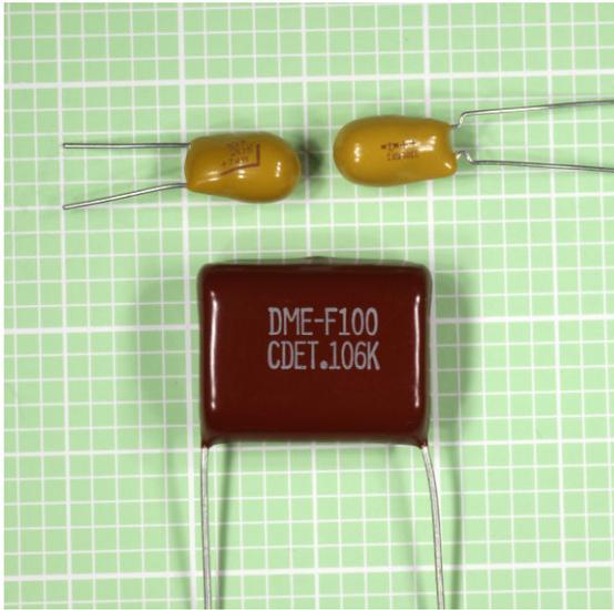
**Figure 12-14.** Two tantalum capacitors are shown above a polyester film capacitor. The polarity of the tantalum capacitors is indicated by the plus signs adjacent to the longer lead, in each case. The polyester capacitor is nonpolarized.
