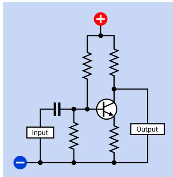
**Figure 28-14.** The basic schematic for a common-emitter amplifier. See text for details.
