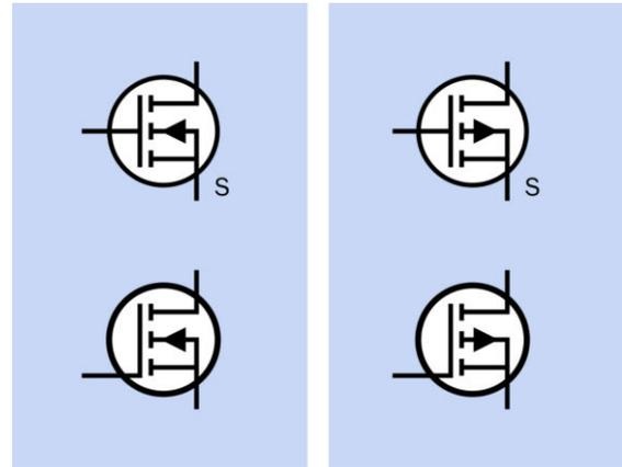
**Figure 29-13.** Schematic symbols for enhancement MOSFETs. The two on the left are functionally identical, and represent N-channel enhancement MOSFETs. The two on the right represent P-channel enhancement MOSFETs.
