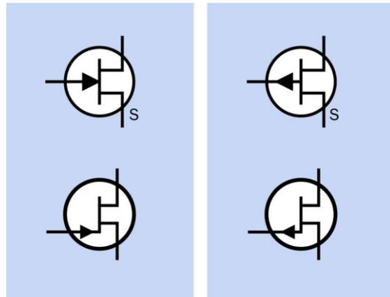
**Figure 29-3.** Schematic symbols for junction field-effect transistors (JFETs). Left: N-channel. Right: P-channel. The symbols at top and bottom on each side are functionally identical. Circles may be omitted. Letter S may be omitted from the symmetrical symbol variants, even though this creates some ambiguity.
