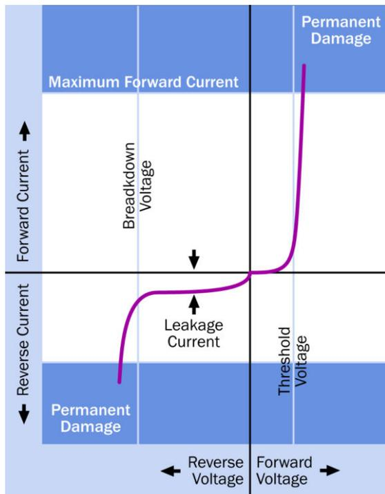
**Figure 26-5.** As the forward voltage across a diode reaches the junction threshold, the diode begins passing current. If the voltage across the diode is reversed, initially a small amount of current leakage occurs. Excessive forward or reverse voltage will create sufficient current to destroy the component.
