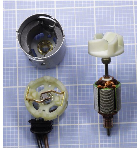
**Figure 22-4.** A traditional DC motor removed from its cylindrical casing. The brushes of the motor are attached to the white plastic end piece at bottom-left. Large squares on the graph paper in the background are 1" × 1", divided in 0.1" increments. The motor was used in a small bilge pump.
