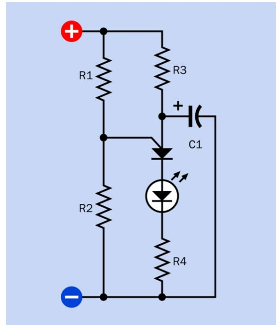
**Figure 27-9.** A basic oscillator circuit using a programmable unijunction transistor (PUT). As the capacitor accumulates charge, the voltage on the anode increases until it triggers the PUT, at which point the capacitor discharges through the anode. The gate voltage is preset by R1 and R2 to adjust the triggering voltage.
