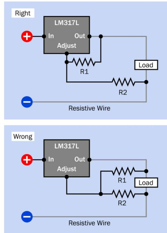
**Figure 19-7.** When the connection between an adjustable-output voltage regulator and load components has a significant resistance (shown here as a gray "resistive wire"), R1 should always be connected as closely as possible to the pins of the regulator, as shown in the upper schematic. (Derived from schematics prepared by National Semiconductor.)
