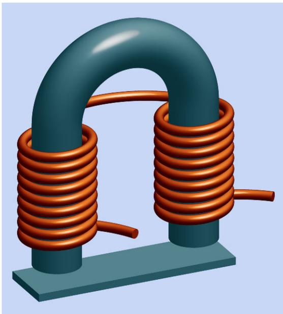
**Figure 20-3.** This traditional design for an electromagnet has a pedigree stretching back for more than a century. It maximizes efficiency by completing a magnetic circuit through any object that the magnet attracts.
