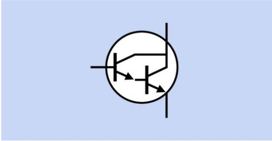
**Figure 28-9.** When a Darlington pair is embedded in a single transistor-like package, it may be represented by this schematic symbol. The leads attached to the package can be used as if they are the emitter, base, and collector of a single NPN transistor.
