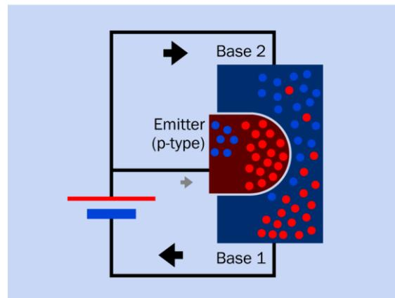
**Figure 27-4.** Internal workings of a unijunction transistor.
