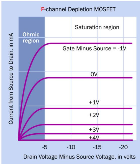
**Figure 29-17.** Current flow through a depletion-type, P-channel MOSFET.
