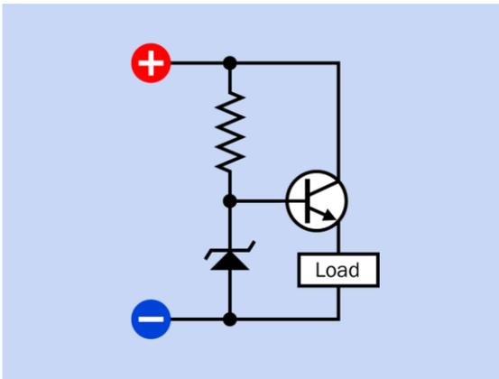
**Figure 26-20.** A transistor could be added to the circuit in the previous figure to reduce power waste through the resistor.
