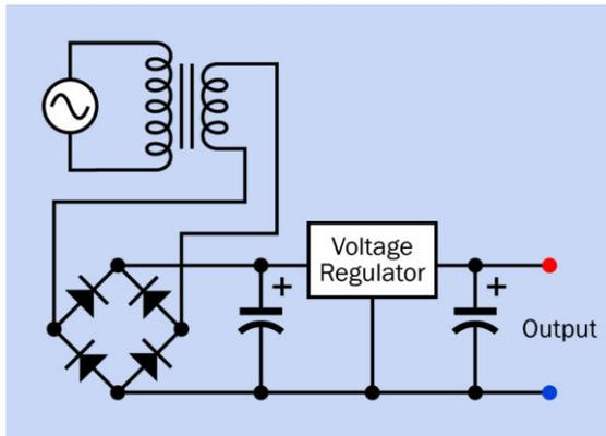
**Figure 16-1.** A basic linear regulated power supply.
