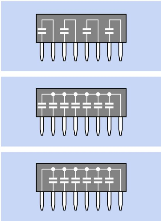
**Figure 12-9.** A *capacitor network* most often consists of a single-inline package (SIP) chip containing multiple capacitors in one of three configurations shown here. Top: Isolated. Center: Common bus. Bottom: Dual-ended common bus. Individual capacitor values ranging from  $0.001\mu\text{F}$  to  $0.1\mu\text{F}$  are common.
