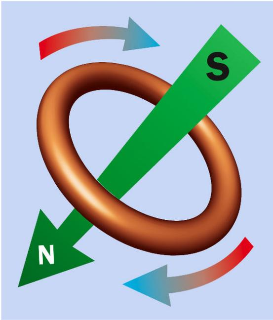
**Figure 14-5.** Hypothetically, if conventional current flows around a circular conductor (as suggested by the red/blue arrows), it will create a magnetic field that can create a force as shown by the green arrow.
