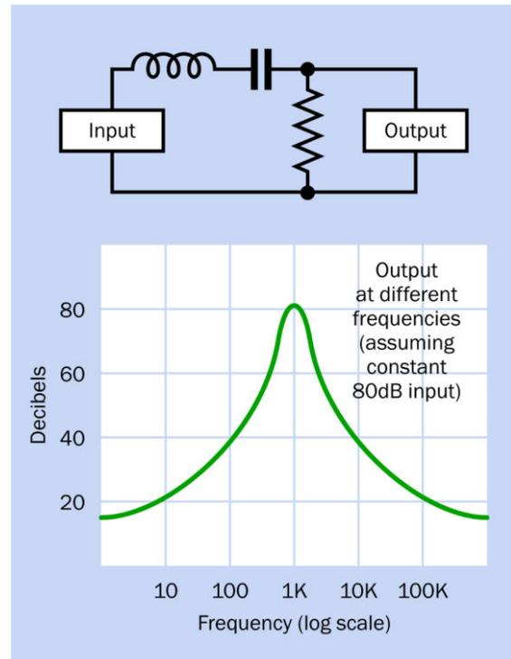
**Figure 14-24.** If the values of a capacitor and an inductor are correctly chosen, and the components are placed in series, the inductor blocks high frequencies while the capacitor blocks low frequencies, creating a bandpass filter, in which only a narrow band of frequencies can get through.
