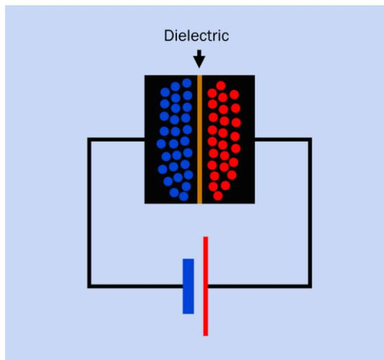
**Figure 12-2.** Because the plates of a capacitor are electrically conductive, they will become populated with positive and negative charges when connected with a DC power source. As opposite charges attract each other, they will tend to congregate on either side of the dielectric, which is an insulating layer. The battery symbol is shown here colored for clarity.
