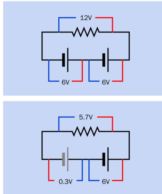
**Figure 2-16.** When a pair of 6V batteries is placed in series to power a resistive load, if one of the batteries discharges completely, it becomes a load instead of a power source, and will be subjected to reverse charging, which may cause permanent damage.
