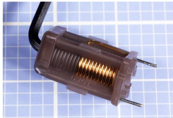
**Figure 14-12.** A variable inductor. Its inductance is adjusted via a screw thread that varies the insertion of the core in the coil. In this component the core is turned by inserting a hex wrench, as shown. It is rated from 0.09 $\mu$ H to 0.12 $\mu$ H.
