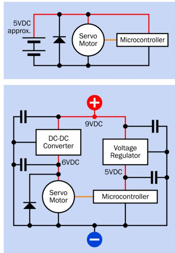
**Figure 24-7.** Two possible schematics to run a small servo motor, the upper example using battery power (for example, from four 1.2V NiMH cells) and the lower example using a 9VDC AC adapter. See text for additional explanation.
