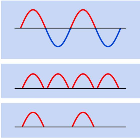
**Figure 26-10.** Top: The voltage-amplitude sinewave of an alternating current source that fluctuates between positive voltage (shown red) and negative voltage (shown blue) relative to a neutral (black) baseline. Center: AC current converted by a full-wave rectifier. Because the diodes do not conduct below their threshold voltage, small gaps appear between pulses. Bottom: Output from a half-wave rectifier.
