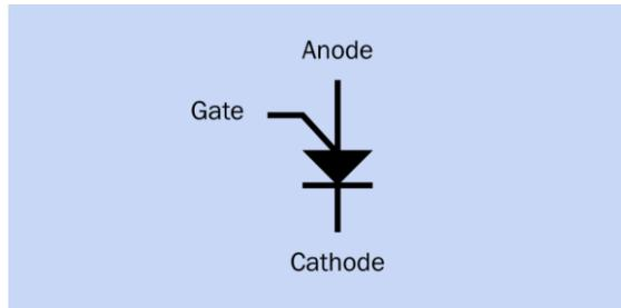
**Figure 27-2.** Schematic symbol for a programmable unijunction transistor (PUT). The symbol accurately suggests the similarity in function to a diode, with the addition of a gate to adjust the threshold voltage.
