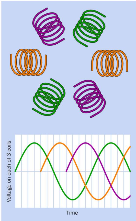
**Figure 23-11.** The graph shows voltage delivered via three wires constituting a three-phase power supply. (The curve colors are arbitrary.) A three-phase motor contains a multiple of three coils—often six, as shown here diagrammatically. The three wires of the power supply are connected directly to the coils, which induce a rotating magnetic field.
