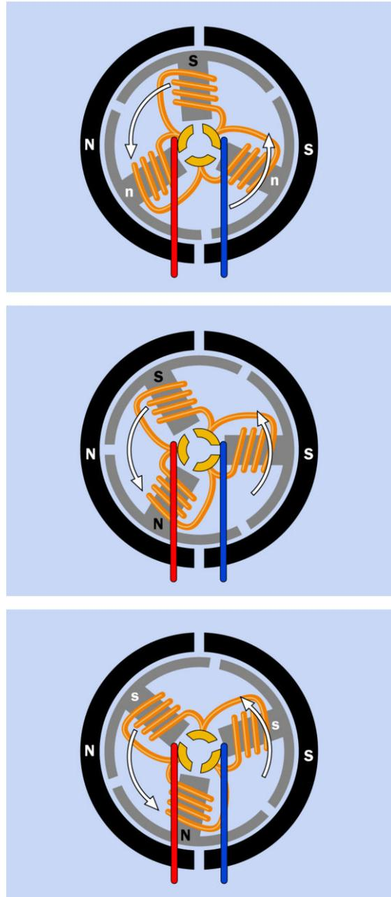
**Figure 22-2.** Three sequential views of a typical three-coil DC motor viewed from the end of its shaft (the shaft itself is not shown). Magnetic effects cause the rotor to turn, which switches the current to the coils via the commutator at the center.
