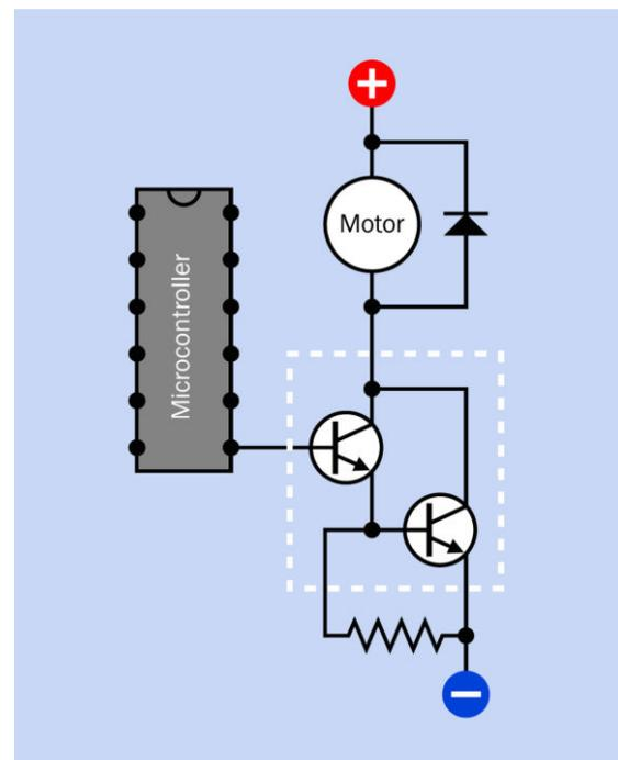
**Figure 28-8.** Where the emitter of one NPN transistor is coupled to the base of another, they form a *Darlington pair* (identified by the dashed rectangle in this schematic). Multiplying the gain of the first transistor by the gain of the second gives the total gain of the pair.
