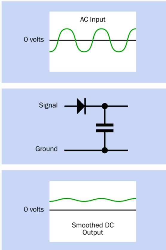
**Figure 12-23.** A capacitor of  $100\mu\text{F}$  or more smooths the upper half of an AC signal that has passed through a diode. The capacitor charges during each positive pulse and discharges to “fill the gaps” between them.
