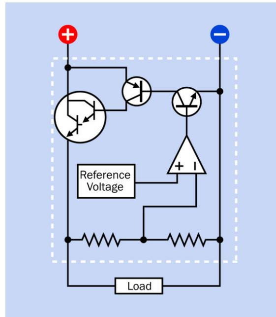
**Figure 19-3.** The fundamental internal features of a standard-type voltage regulator, including a Darlington pair, two transistors, a voltage divider, comparator, and reference voltage source, shown inside the dashed white line.
