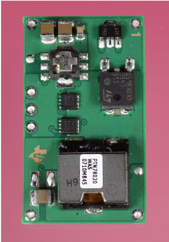
**Figure 17-9.** Another adjustable DC-DC converter. The output voltage is determined by adding an external resistor or trimmer potentiometer. External smoothing capacitors are required, as shown in the component's datasheet.
