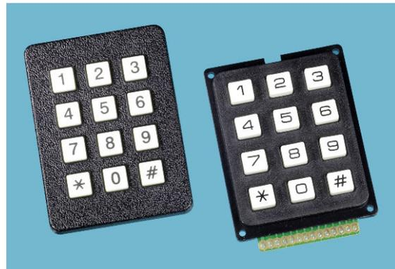
**Figure 5-12.** The keypad on the left is matrix-encoded, and is polled via seven through-hole pins that protrude behind it. The keypad on the right assigns each button to a separate contact in its header. See the text for details about matrix encoding.
