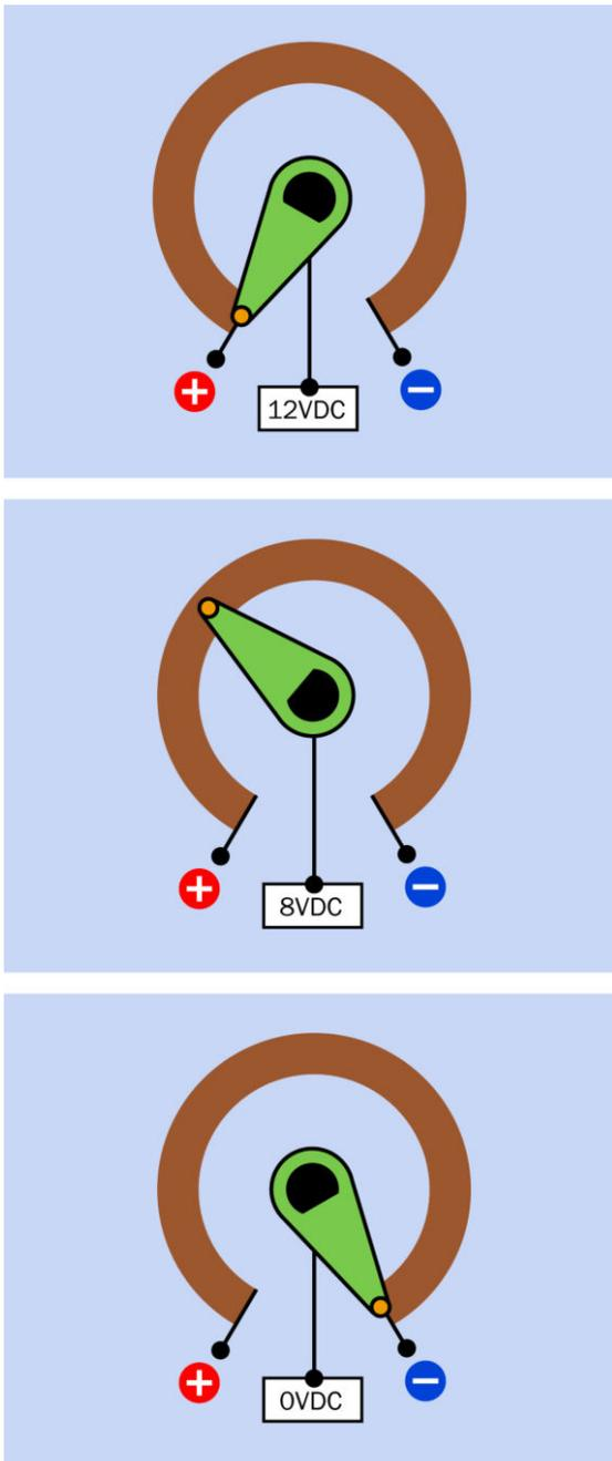
**Figure 11-3.** Inside a potentiometer. See text for details.
