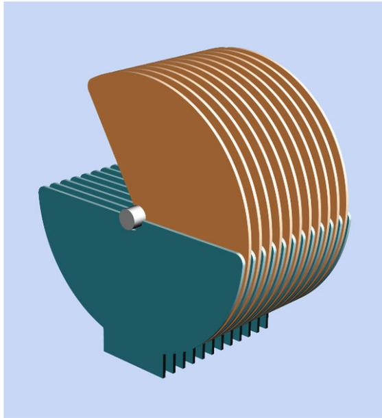
**Figure 13-2.** In this simplified view of a variable capacitor, the brown plates constitute the rotor, attached to a central shaft, while the blue plates are the stator. The colors have no electrical significance and are added merely for clarity. The area of overlap between rotor and stator determines the capacitance.
