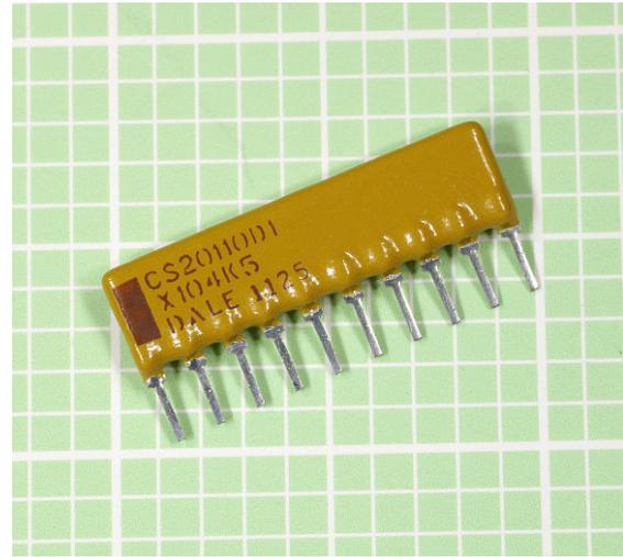
**Figure 12-10.** A capacitor array in through-hole, SIP format.
