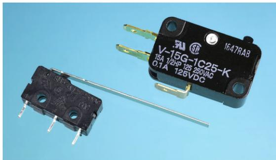
**Figure 6-4.** Two SPDT snap-action switches, also known as limit switches. The one on the right is full-size. The one on the left is miniature, with an actuator arm to provide additional leverage. The arm may be trimmed to the required length.
