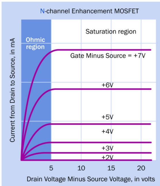
**Figure 29-18.** Current flow through an enhancement-type, N-channel MOSFET.
