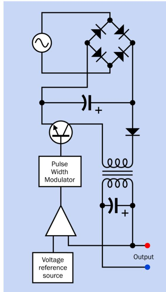
**Figure 16-4.** Greatly simplified schematic showing the principal components of a switching power supply. Note the absence of a 115VAC power transformer. The transformer that is inserted subsequently in the circuit functions in conjunction with the high switching frequency, which allows it to be very much smaller, cheaper, and lighter.
