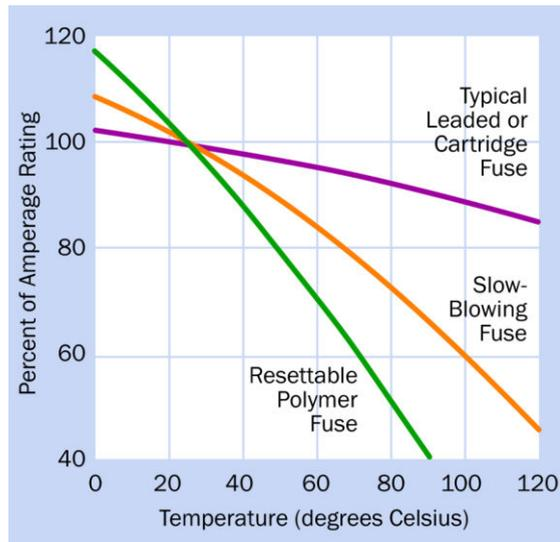
**Figure 4-10.** The three curves give a very approximate idea of the temperature sensitivity of three types of fuses commonly used to protect electronic equipment. The left-hand scale provides an approximate value for the amperage which will trip the fuse.
