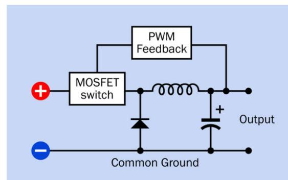
**Figure 17-3.** Basic topology of a buck-type DC-DC converter.
