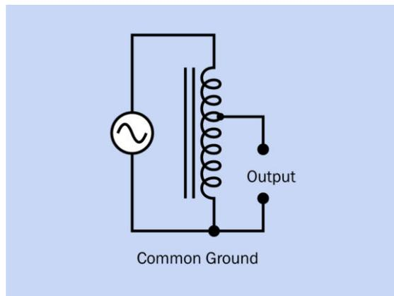
**Figure 15-10.** An autotransformer contains only one coil and core. A reduced output voltage can be obtained by tapping into the coil. A common connection prevents the output from being electrically isolated from the input.
