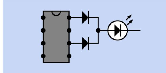
**Figure 26-18.** Two or more outputs from a logic chip or microcontroller may be coupled with diodes to power another device, such as an LED, while protecting the chip from backflow of current. The diodes form a logical OR gate.
