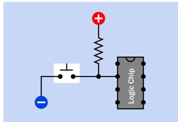
**Figure 10-17.** A pulldown resistor (top) or pullup resistor (bottom) prevents an input pin on a logic chip or microcontroller from “floating” in an indeterminate state when the button is not being pressed.
