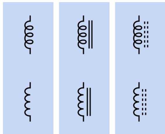
**Figure 14-1.** The coil symbol for an inductor may be drawn in two styles which are functionally identical. Line(s) beside the coil indicate a solid core. Dotted line(s) indicate a core containing metal particles.
