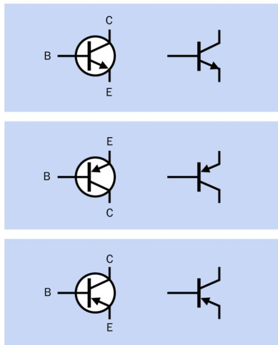
**Figure 28-1.** Symbols for an NPN transistor (top) and a PNP transistor (center and bottom). Depending on the schematic in which the symbol appears, it may be rotated or inverted. The circle may be omitted, but the function of the component remains the same.
