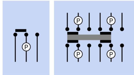
**Figure 5-6.** Left: schematic symbol for a simple SPDT slide pushbutton, where a movable contact shorts together either the left pair or right pair of fixed contacts. Right: A 4PDT pushbutton in which the same principle has been extended. The movable contacts are attached to each other mechanically by an insulator. Each pole terminal is marked with a P.
