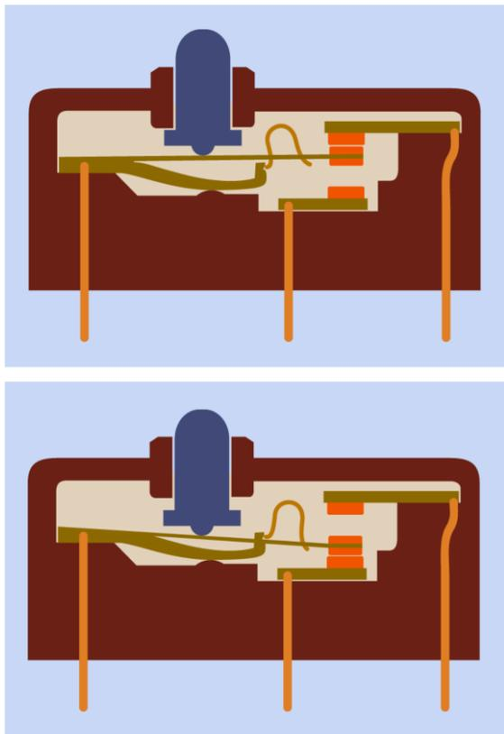
**Figure 6-5.** Top: Two contacts inside this limit switch are touching by default. Bottom: When the external button is pressed, it pushes a flexible metal strip downward until it connects with the lower contact. The inverted-U-shaped component is a spring that rests inside a cutout in the flexible strip and resists motion through the central part of its travel.
