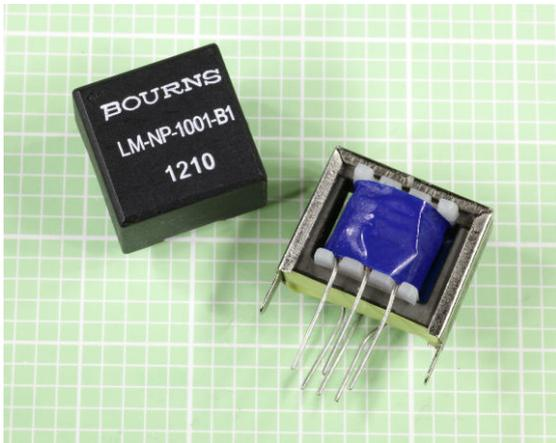
**Figure 15-12.** Through-hole transformers. See text for details.
