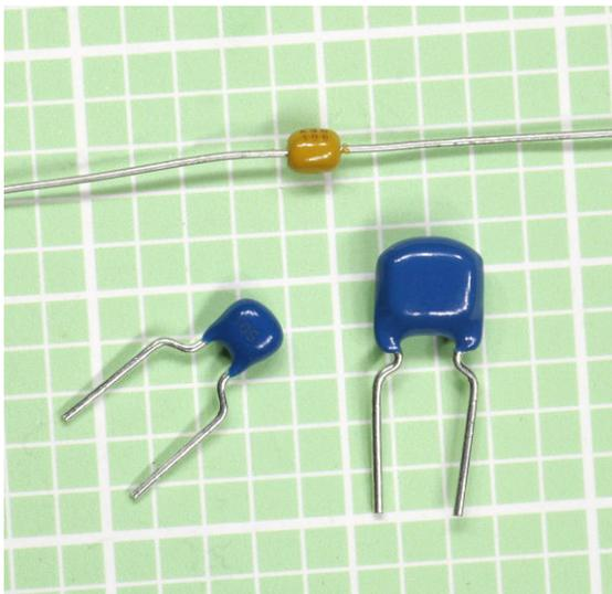
**Figure 12-15.** Multilayer ceramic capacitors are extremely compact, and are nonpolarized. Top:  $1,000\text{pF}$  (i.e.  $1\text{nF}$ ) at  $100\text{V}$ . Bottom left:  $1\mu\text{F}$  at  $25\text{V}$ . Bottom right:  $47\mu\text{F}$  at  $16\text{V}$ .
