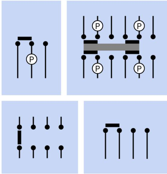
**Figure 6-9.** Slide switch schematics. Each black rectangle represents a movable contact that connects two pairs of fixed contacts at a time. Detailed commentary on these variants will be found in the body of the text. Manufacturers may use variants of these symbols in their datasheets (for example, the gray rectangle indicating an insulating contact carrier, at top right, may be represented as a single line, or a black outline with a white center).
