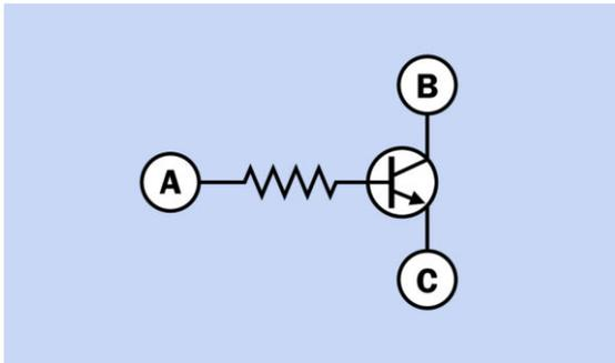
**Figure 10-16.** A resistor is typically necessary to protect the base of a transistor from excessive current.
