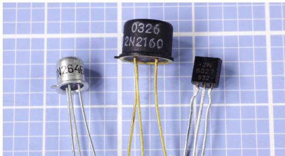
**Figure 27-3.** The unijunction transistors at left and center are becoming obsolete; the one at the right is a programmable unijunction transistor (PUT), still readily available and widely used as a thyristor trigger.
