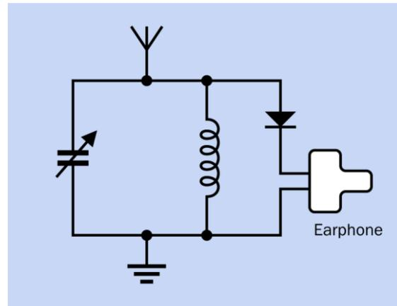
**Figure 13-6.** The principle of an LC circuit is used here in a basic circuit that can tune in to a radio station and create barely audible sound through the earphone at right, using only the broadcast signal for power. The variable capacitor adjusts the frequency of the circuit to resonate with the carrier wave of the radio signal.
