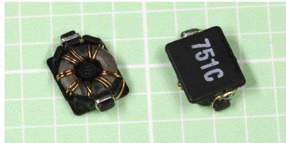
**Figure 14-14.** In a typical toroidal inductor, the coil is wrapped around a magnetic core shaped as a torus. This surface-mount component (viewed from the bottom, at left, and from the top, at right) is at the low end of the range of component sizes. It is rated at  $750\text{nH}$ .
