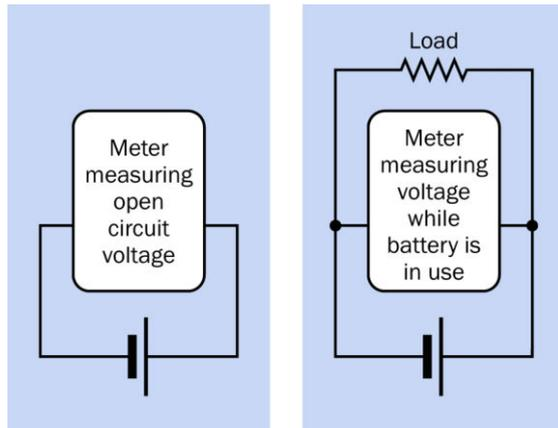
**Figure 2-13.** When using a volt meter (or a multimeter configured to measure voltage), the meter can be applied directly between the battery terminals to determine the open-circuit voltage (OCV), or in parallel with a load to determine the voltage actually supplied during use. A multimeter must be set to measure DC volts before connecting it across a battery. Any other setting may damage the meter.
