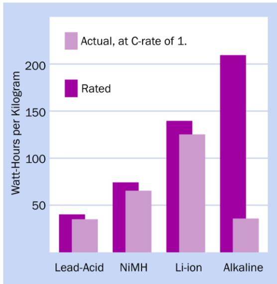
**Figure 2-6.** Because of their relatively high internal resistance, alkaline batteries are especially unsuited to high discharge rates, and should be reserved for applications where a small current is required over a long period. (Chart derived from <http://batteryuniversity.com>.)
