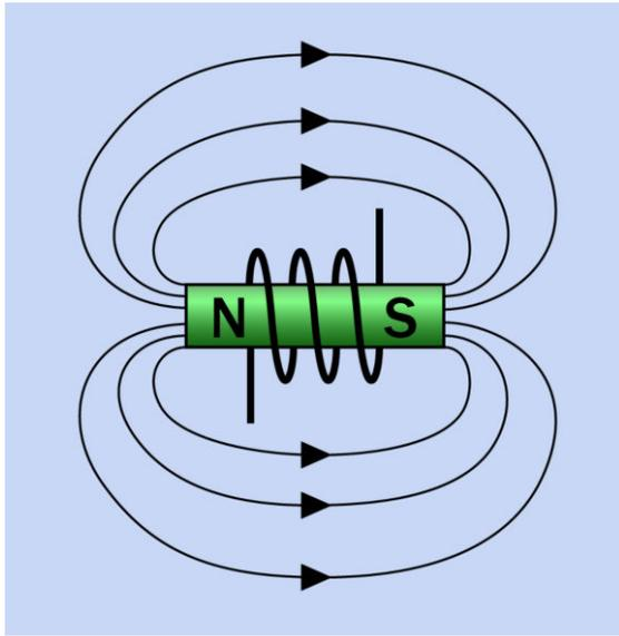
**Figure 14-7.** A magnetic field in reality is not open-ended, and each line of force traveling through a rod-shaped magnet or electromagnet is completed outside of the magnet. The completion of magnetic fields has been omitted from other diagrams here for clarity.
