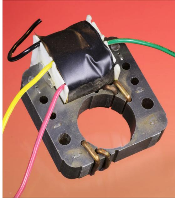
**Figure 23-3.** This stator from a smaller electric fan uses only a single coil, wrapped in black tape. It is sufficient to induce a magnetic field but is generally less efficient than a motor using multiple coils.
