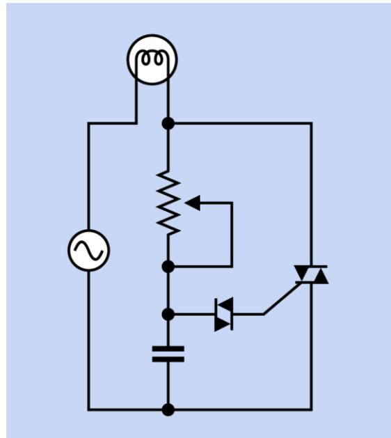
**Figure 11-10.** Typical usage of a potentiometer in conjunction with a diac, triac, and capacitor to control the brightness of an incandescent bulb, using an AC power supply. Diacs and triacs are discussed in Volume 2.
