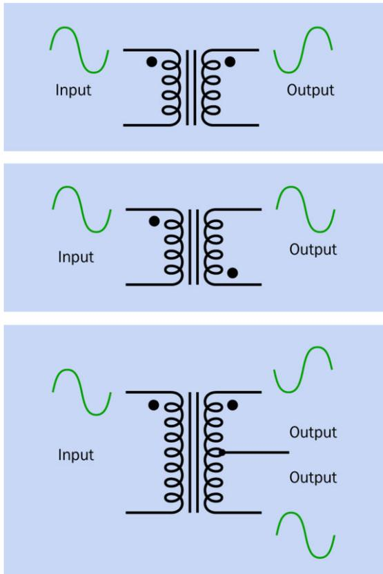
**Figure 15-7.** A dot indicates the start of each winding. Where primary and secondary windings are in the same direction, the voltage output will be 180 degrees out of phase with the input. Where the dots indicate windings in opposite directions, the voltage output will have the same phase as the input. Where a center tap on the secondary winding serves as a common ground, the voltages at opposite ends of the secondary winding will be opposite to each other in phase.
