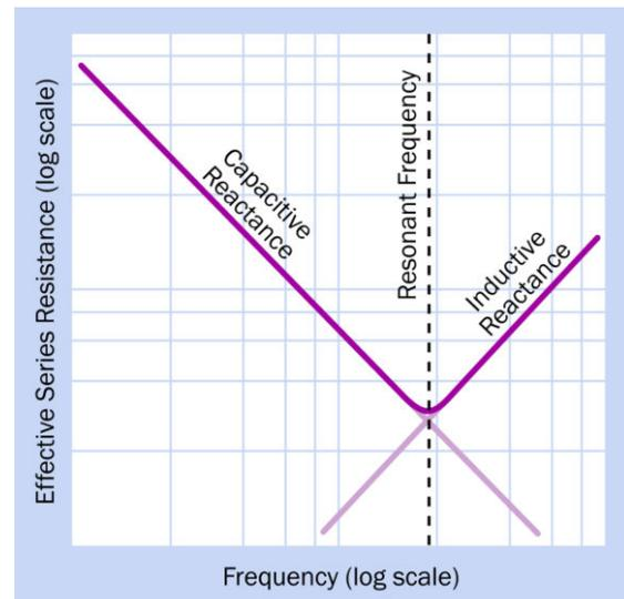
**Figure 12-18.** As an AC current applied to a capacitor increases in frequency, the *capacitive reactance* of the component decreases, while its *inductive reactance* increases. The resonant frequency of the capacitor is found where the two functions intersect.
