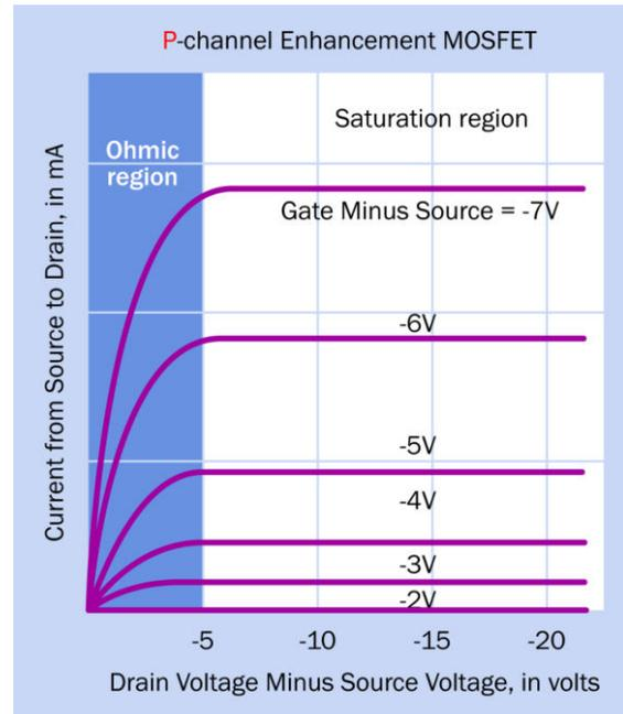
**Figure 29-19.** Current flow through an enhancement-type, P-channel MOSFET.
