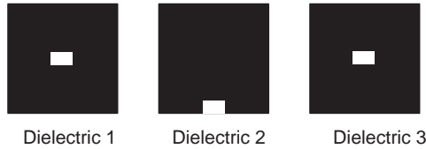
Figure 9.16 Masks for dielectric layers.
