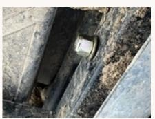
Begin reinstalling the skid plate loosely.(You may need to clean the dirt out of the plastic channels behind the plastic trim.)
