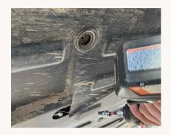
Place your tree-kickers up to the body and install the bolts with a washer on each side, through the frame holes and loosely install the nylock nuts. (The lower rear bolts are the hardest because of a factory gusset. Here you will need to use needle nose pliers or a magnet to hold the nut up in place to start the bolt. Each machine is different and some grinding on the gusset may be necessary.)
