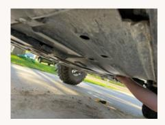
up front and 2 square holes in rear in place, you can tighten the skid plate bolts back down. Make sure the washers line up with the holes on the skid plate when tightening them back down. If they don't, you may need the rubber mallet to persuade the skid plate to move a little bit to line them up.
