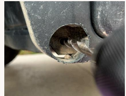
**2** Using a 7/16" drill bit, drill out the 4 factory holes.
