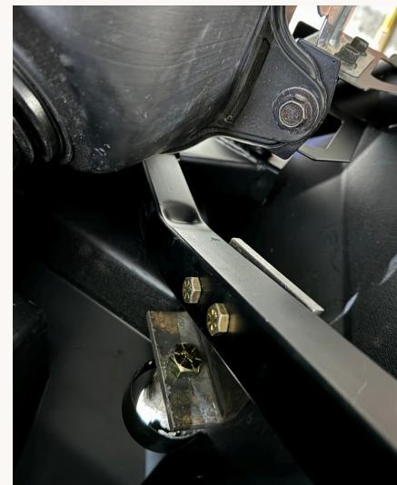
**6** Tap the bolt into place. On the Bruiser Series, the rear mount on the Driver's Side, you will have to tap the bolt by the fuel tank, and this can be done by using a floor jack and putting a little pressure on the fuel tank. (The bolt head might rub the fuel tank some, each vehicle is different.)
