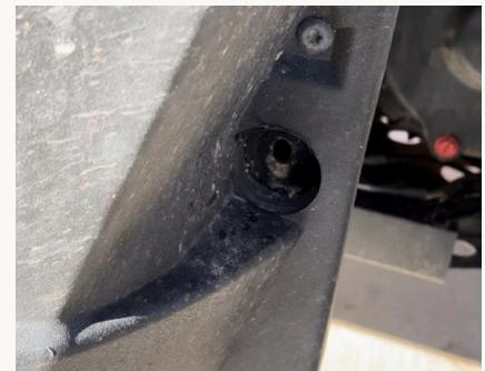
**3** Remove the lower rear T40 torx bolt off the frame (in front of rear wheels) and drill a 7/16" hole all the way through the frame. Clean up inside of frame with file so bolt sleeve fits in frame.
