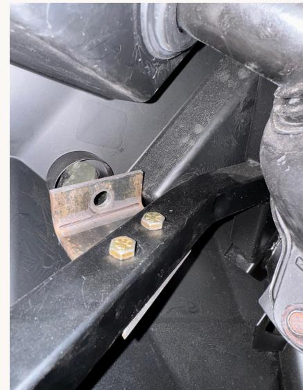
**5** On our Step Series, Double Barrel & Basic Series, the 3/4" x 6" & 6-1/2" Bolts will go in from the front side, through the slider, & through the frame, with a Nylock Nut on the back side. On the Bruiser Series, the bolt has to go in from the back side, and the Nylock Nut on the outside of the slider.
