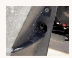
Mount sliders in body and use Floor Jack to support the sliders (or have another person hold them in place). Install the upper rear bolt with a washer (longest one of the long bolts) and put washers and nut on finger tight to hold in place (if you do not have jack stands or a helper).
