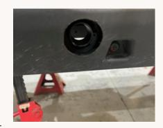
Place your new tree kickers/sliders onto the bolts, and using the 5/8" washers and tin 5/8" nylock nuts to hold them into place, get everything lined up and tighten the 5/8" nylock nuts.
