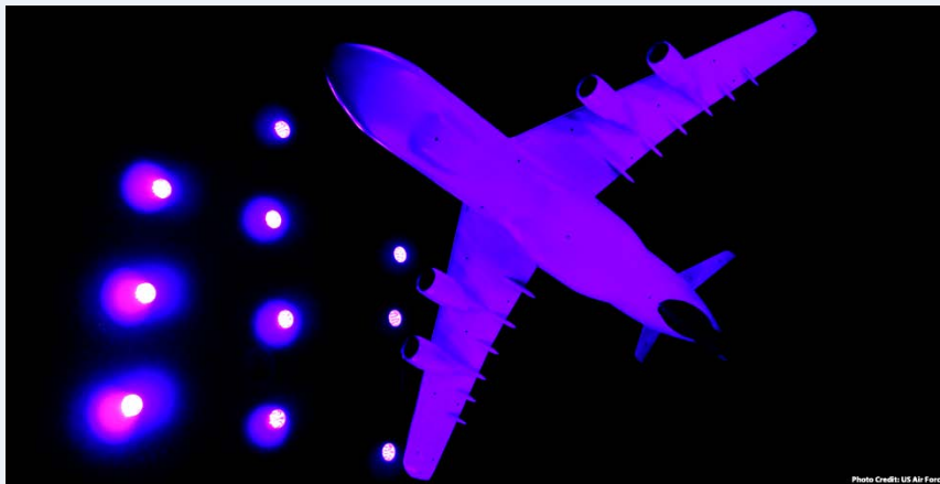
ISSI LEDs Mounted in AEDC 16T Wind Tunnel, Photo Credit US Air Force (Left), ISSI LEDs Mounted in NASA Ames Research Center 11'x11' TWT (Credit: D. Hart / NASA Ames Research Center)
