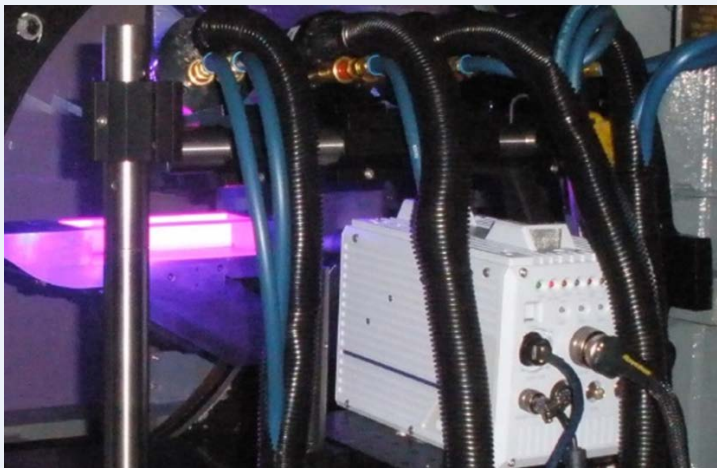
ISSI LEDs Mounted in Cavity Acoustics Fast PSP Test (Left), Courtesy US Air Force Research Laboratory, ISSI Water-Cooled LEDs mounted in a Fast PSP Turret Test (Right), Courtesy of Stanislav Gordeyev, AME Dept, University of Notre Dame
