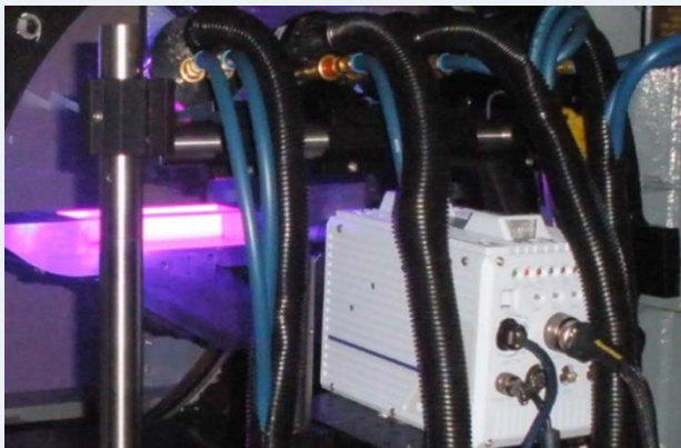
Fast PSP in a Subsonic Cavity Under UV Excitation (Left), Standing Pressure Waves in a Subsonic Cavity (Right), (Courtesy: US Air Force)
