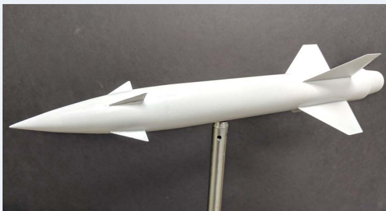
(Left) Epoxy Screen Layer Part A (White) and Part B (Yellow/clear), (Right) Missile Model Painted with Screen Layer
