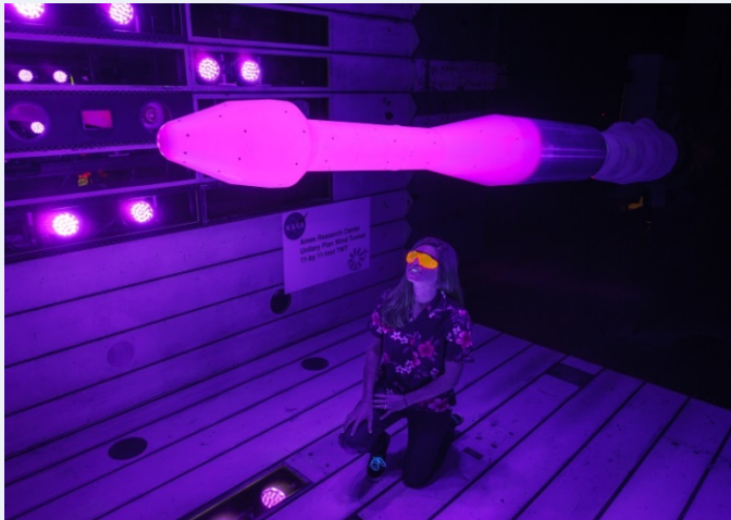
Fast PSP Under UV Excitation on a Space Launch Vehicle Model (Left), Processed Unsteady Pressure Fluctuations from Buffeting at 6.10 Hz (Right), (Credit: D. Hart / NASA Ames Research Center)
