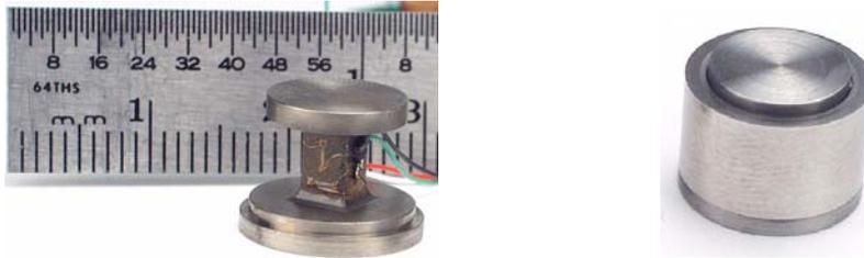
The subminiature load cells above are shown with and without a protective sleeve. The typical combined error due to nonlinearity and hysteresis is less than 0.1% of the full scale output. Similar installations can be done on any small mechanical piece where strain measurement is needed.
