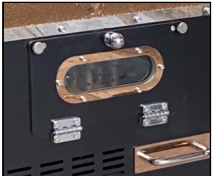
FRONT BURNER ROOM DOOR
