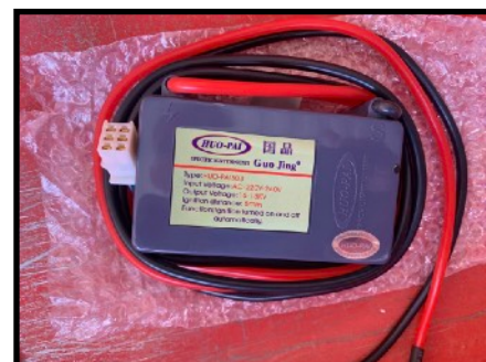
NEW IGNITER SYSTEM AS OF 2024
