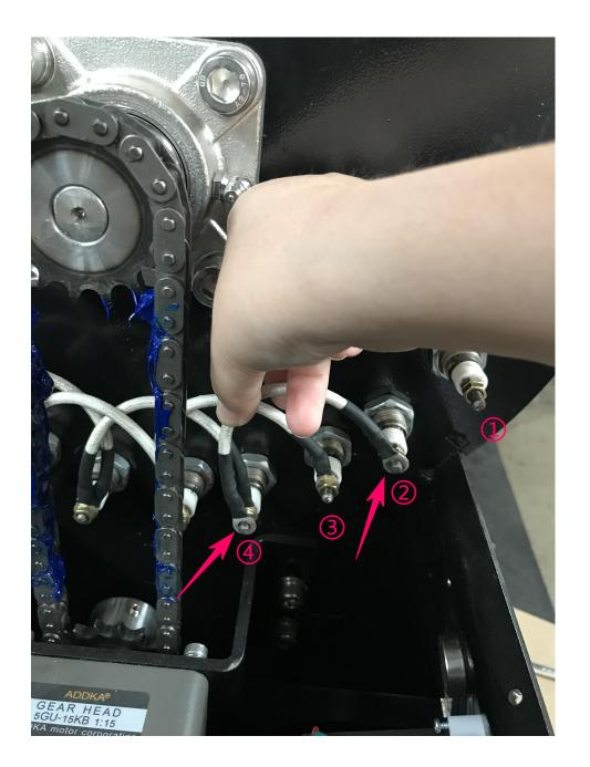
pick up one connection line connect one end with ④ connect the other end with ②
