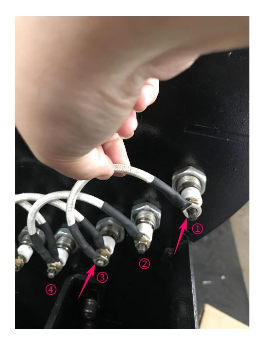
Pick up another connection line connect one end with ③ connect the other end with ①
