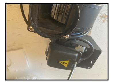
2. THERE YOU WILL FIND THE 2 POWER WIRES GOING INTO FAN ELECTRIC BOX. YOU CAN SNIP THESE OFF BELOW THE CONNECTORS ALLOWING ENOUGH SPARE WIRE TO CONNECT THE 2 POWER WIRES FROM YOUR 3 PRONG CORD TO THESE AND THEN THE 3RD WIRE SHOULD BE THE GROUND WIRE THAT CAN BE ATTACHED TO THE BASE OF FAN INSIDE ELECTRIC BOX USING A SCREW FROM THE OLD FAN TO ATTACH IT TO BASE OF FAN. 1. USING A SCREWDRIVER REMOVE THE COVER OVER THE ELECTRIC BOX ON CHAFF FAN.
