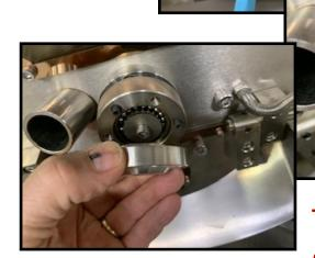
3. Once you have screwed all the set screws into place FIT the cover back over holder and insert the 3 screws that holds cover into place and hand tighten
