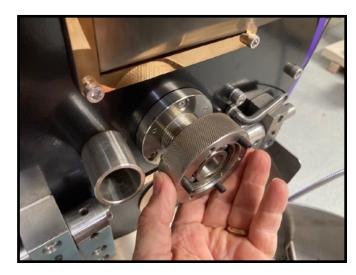
11. IF NEEDED YOU MAP TAP BEARING FURTHER INTO HOLDER IF NOT FULLY INSERTED
