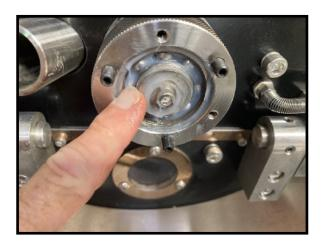
14. REINSTALL COVER & ADJUST SET SCREWS AS NEEDED. THEN RUN ROASTER DRUM IN BOTH COLD AND A HEAT TEST TO
