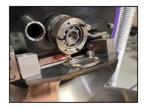
5. AFTER REMOVED PREPARE TO REMOVE OLD BEARING FROM HOLDER BY TAPPING IT OUT
