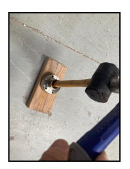
6. SET HOLDER ON A BLOCK OF WOOD AND USING A WOOD HANDLE OR WOOD DOWEL ROD TO TAP OLD BEARING OUT OF HOLDER
