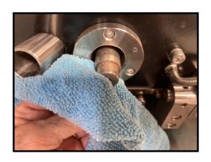
8. CLEAN DRUM SHAFT OF DEBRIS. IF YOU LIKE YOU CAN PUT A THIN COATING OF GREASE ON SHAFT
