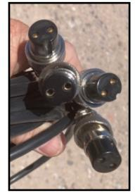
The BC Models use two different size Aviation plugs as well as plugs that are 2 prong and 3 prong as can be seen here:
