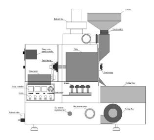
THE BC-3.5 IS A HEAVY DUTY ROASTER BUILT WITH A CARBON STEEL BODY WITH APPROVED POWDER COAT HIGH TEMPERATURE BODY IN BLACK, WHITE OR RED . THE HOUSINGS COME IN SOLID COLOR CHOICES & TEXTURED COLORS. TWO EXHAUST PIPES COMES OFF THE BC-3 AT 3" AS SHOWN BELOW AND CAN BE EXHAUSTED OUT OF BUILDING SEPARATELY OR CONNECTED WITH A BLAST OR BACKDRAFT DAMPER
