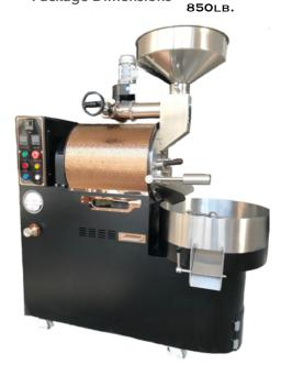
THE BC-8 HD IS A HEAVY DUTY ROASTER BUILT WITH A CARBON STEEL BODY WITH APPROVED POWDER COAT HIGH TEMPERATURE BODY IN BLACK, RED OR WHITE. THE HOUSINGS COME IN A CHOICE OF SEVERAL COLORS.
