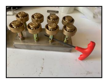
3. ONCE THE STEM AND DIFFUSER IS REMOVED YOU CAN USE A FINE NEEDLE TO POKE THROUGH ORIFICE HOLE TO UNCLOG IT. (DO NOT USE A TOOL THAT COULD ENLARGE ORIFICE HOLE)
