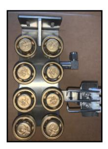
THE BURNER ROOM OF ALL ROASTERS SHOULD BE CLEANED EVERY 3-6 MONTHS OR MORE OFTEN IF NEEDED. TO CLEAN OPEN THE FRONT OR BACK PANEL AND VACUUM OUT ROOM WITH A SHOP VAC AND WIPE DOWN WALLS AND BURNERS TO REMOVE ANY DIRT, DUST AND CARBON BUILDUP
