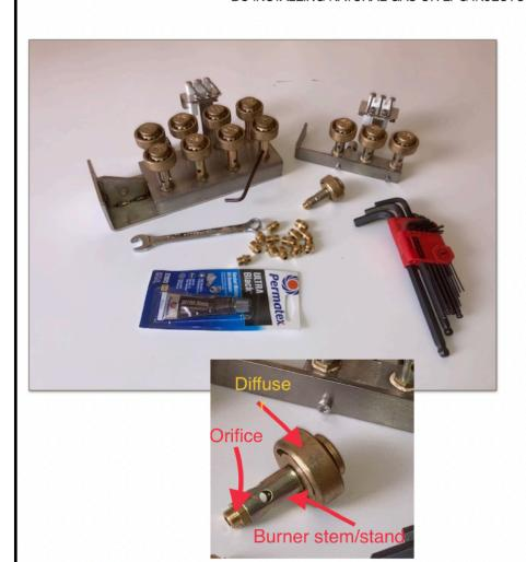
ALL BC ROASTERS COME SETUP WITH LPG (PROPANE) ORIFICES. WHEN USING LPG YOU WILL NEED THE MARSHALL 1912/197 LPG REGULATOR & GAS LINE
