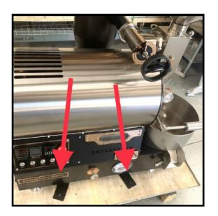
BC-3.5'S & 5'S ARE ATTACHED TO BASE OF CRATE WITH A FEW STEEL BRACKETS. YOU WILL NEED TO USE EITHER A WRENCH OR METRIC HEX KEY (DEPENDING ON BOLT TYPE)
