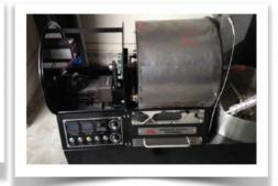
BE SURE TO KEEP MACHINE CLEAN DAILY AND COMPLETELY CLEAN ALL EXTERIOR WEEKLY AND INSIDES OF CHAFF & DEBRIS CONTAINERS ON A REGULAR BASIS. ALWAYS COOL DOWN ROASTER AT END OF DAY BEFORE TURNING OFF.
