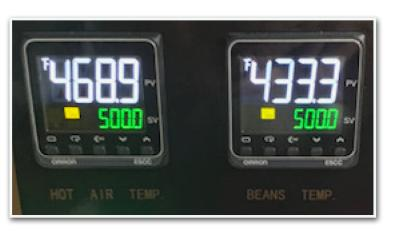
**ELECTRIC CONTROL PANEL:** (Note: On 2018 AND **NEWER MODELS KEEP** THE HOT AIR **ADJUSTMENT FAN ON** 100% AND USE THE MANUAL DIAL DAMPER TO CONTROL AIRFLOW)
