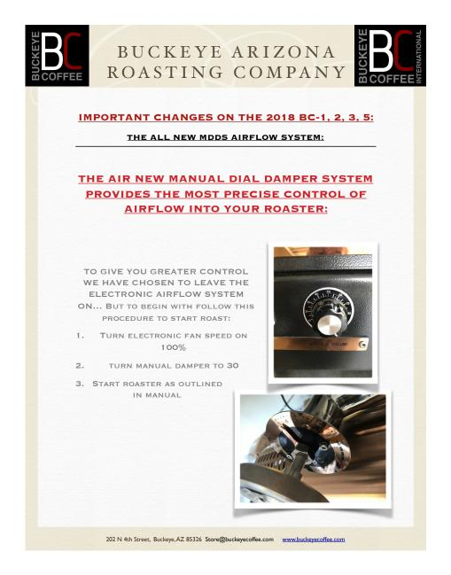
IN 2018 WE ADDED MANUAL DIAL DAMPER SYSTEMS TO MOST ROASTERS SMALLER THAN THE BC-35 AS WE FOUND THE STEPLESS AIRFLOW CONTROLLER WAS NOT A VERY ACCURATE SYSTEM FOR AIRFLOW. ON THE BC-2 MODEL AS OF 2022 AND THE BC-3-5 MODELS FROM 2018 TO 2021 WE LEFT THE AIR VOLUME CONTROL KNOB (HOT AIR VOLUME ADJUSTMENT KNOB) ON CONTROL PANEL TO ALLOW YOU TO TURN OFF THE FAN SPEED WHILE EMPTYING CHAFF UNIT)
