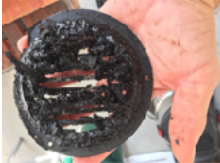
CHAFF FAN RUINED DUE TO FAILURE TO MAINTAIN IT IMPROPER OR NO MAINTENANCE WILL CAUSE FIRE HAZARDS & DESTROY EQUIPMENT
