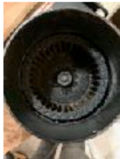
CHAFF FAN RUINED DUE TO FAILURE TO MAINTAIN IT IMPROPER OR NO MAINTENANCE WILL CAUSE FIRE HAZARDS & DESTROY EQUIPMENT
