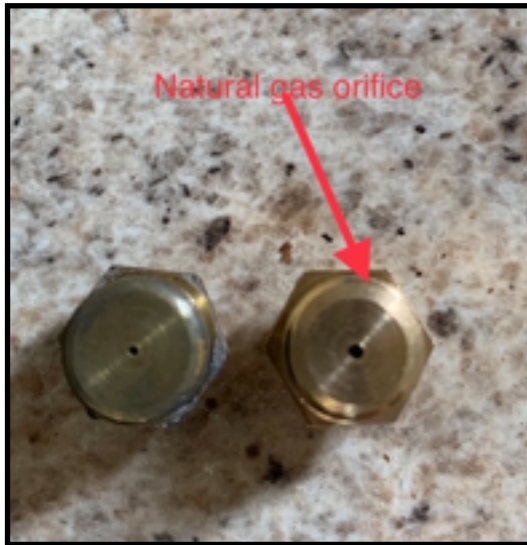
IMAGE: LEFT: LPG ORIFICE RIGHT: NATURAL GAS ORIFICE
