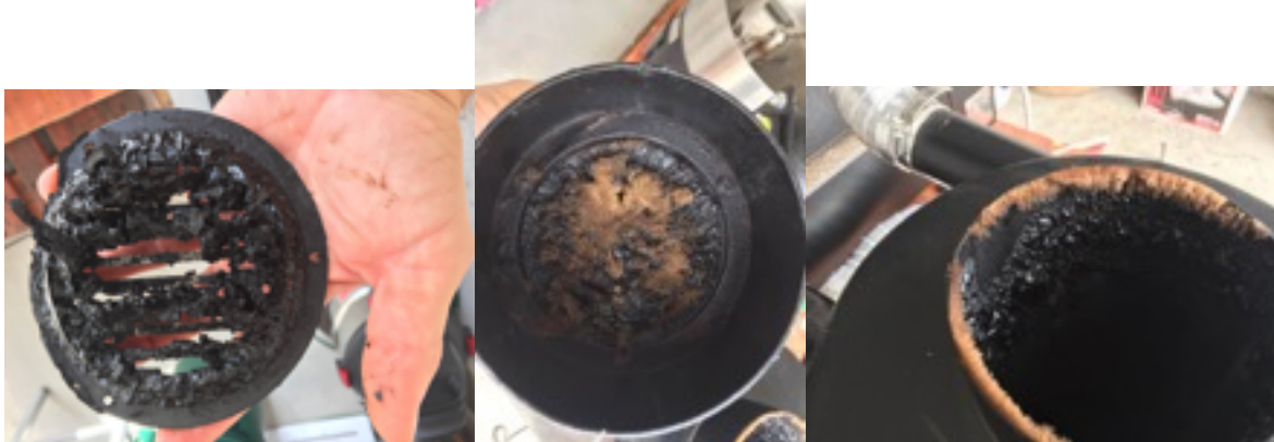
EXAMPLES OF EQUIPMENT RUINED BY NOT CLEANING FAN, VENTING & CHAFF UNIT
