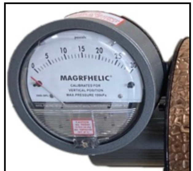
ALL BC ROASTERS OFFER THE MAG AIRFLOW CONTROL GAUGE
