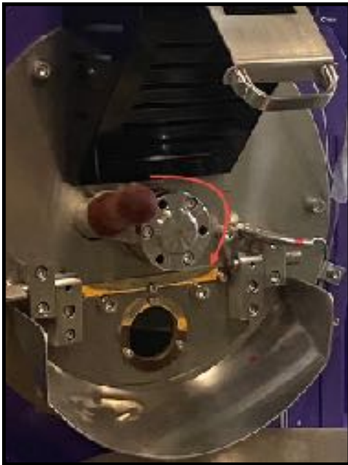
TURNING BEARING HOLDER CLOCKWISE PULLS DRUM AWAY FROM FRONT PLATE
