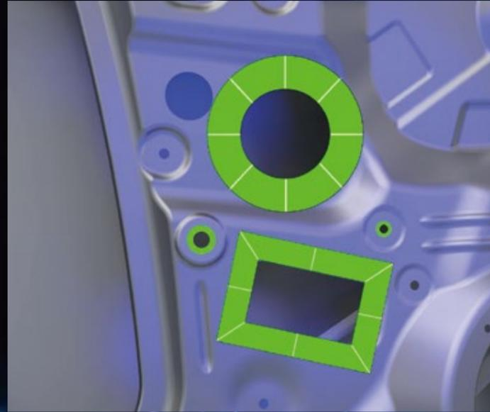
It boasts a shadow-less-light edge detection with high-precision gray value measurement. Users can inspect closed features precisely, especially threaded holes. Good measurements are ensured by delivering accurate and repeatable measurement results such as positions and diameters.
