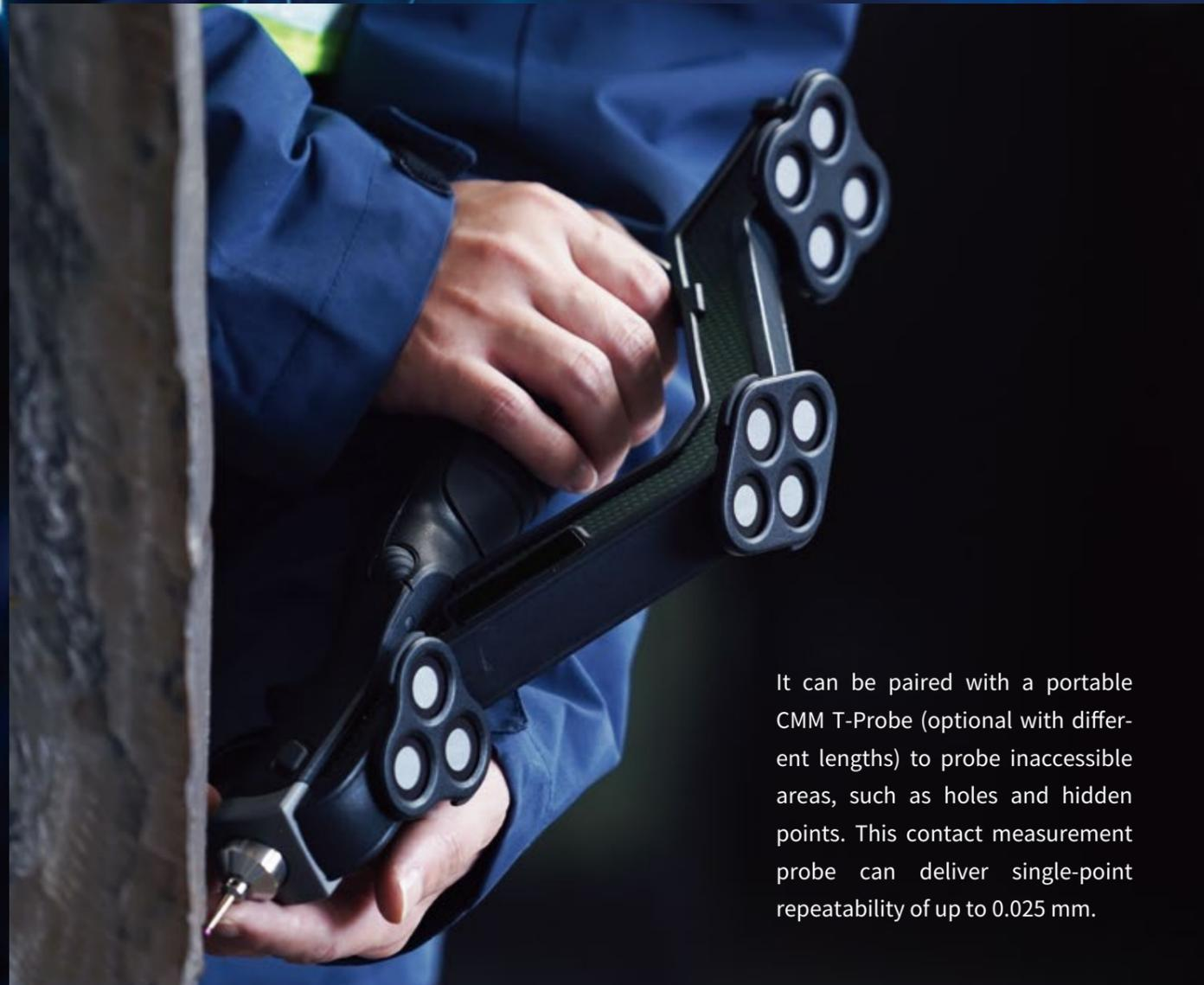
It can be paired with a portable CMM T-Probe (optional with different lengths) to probe inaccessible areas, such as holes and hidden points. This contact measurement probe can deliver single-point repeatability of up to 0.025 mm.
