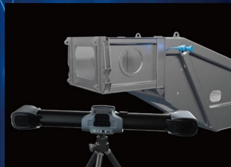
Its i-Tracker can be combined with tool simulators and path planning software to form M-Track, an intelligent robotic path planning and guiding system. The system comprises perception, planning, and execution modules, which cater to different applications such as grinding, coating, welding, and more.
