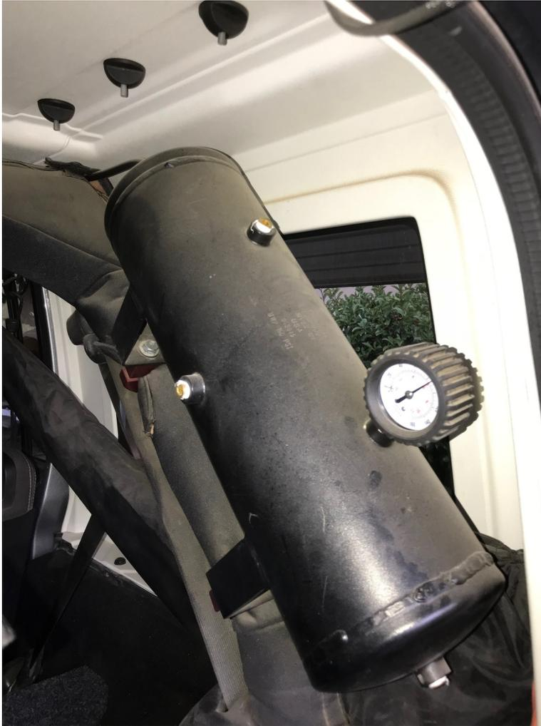
the compressor from working so hard. When used in conjunction with an air pressure shut off valve, once the reservoir tank reaches the set pressure, the compressor turns off - letting it rest (even as you move from one tire to the next). Second, the reservoir allows for more efficient and constant use of air tools. It minimizes the pulsation in the system caused by a reciprocating compressor. Third, the tank allows the air to cool prior to delivery.
