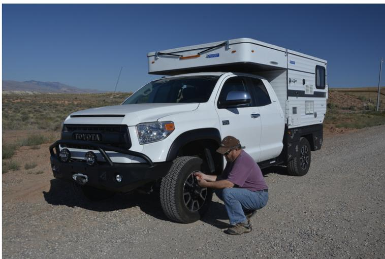
You should always air down your tires when traveling off-road. Once you return to the pavement, you must air them back up to proper highway operating pressures (with few exceptions these pressures are found on the driver's
