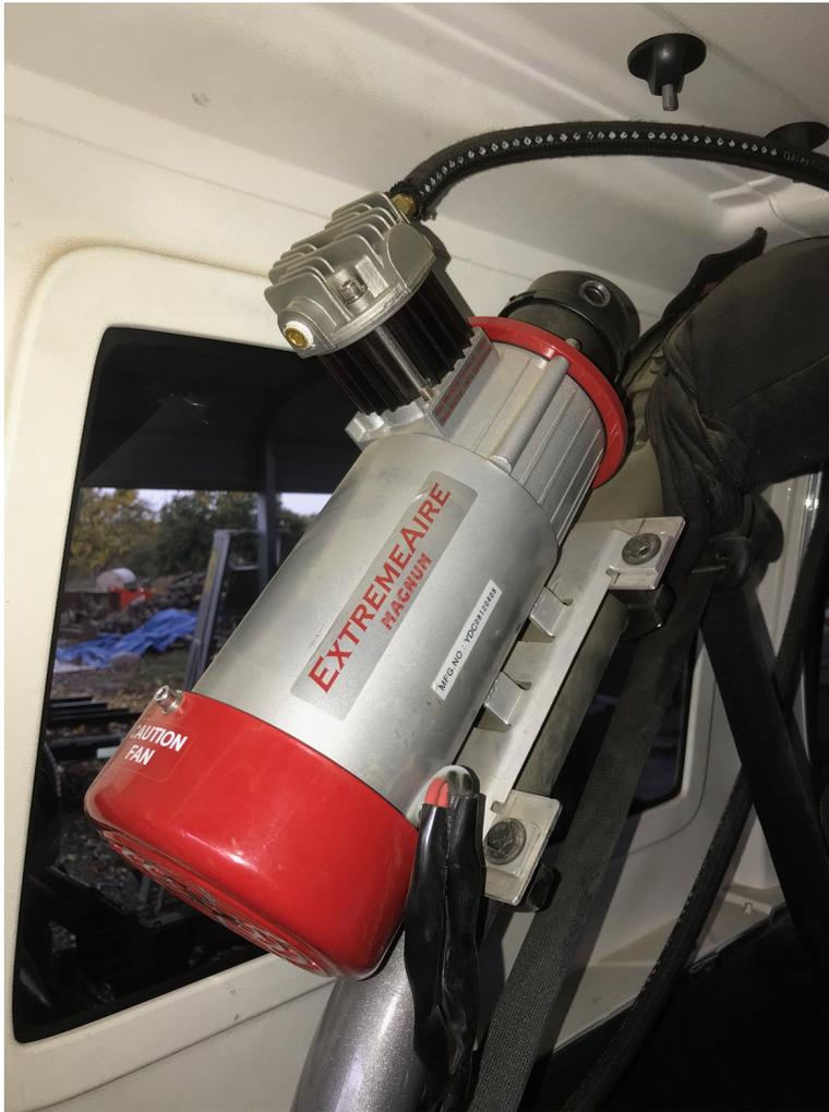
protected areas. Some compressors come with specific vehicle mounting plates and hardware, while other options can be purchased through aftermarket companies. Permanent mounting solutions can also incorporate a small tank, permitting the use of air tools and faster tire fill times. Those that have air-activated lockers often have permanently mounted 12-volt compressors, serving double duty – engaging the lockers and re-inflating tires.
