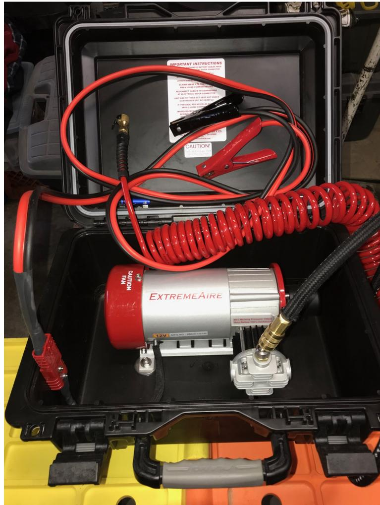
**Extreme Outback Products Compressor.** The compressor shown here is, in my opinion, the best portable compressor made. It has heavy-duty EVERYTHING - box, battery clamps, heat dissipating hose, coiled air hose, super chuck, Plano water proof and dust proof box.
