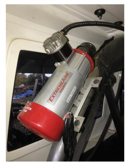
protected areas. Some compressors come with specific vehicle mounting plates and hardware, while other options can be purchased through aftermarket companies. Permanent mounting solutions can also incorporate a small tank, permitting the use of air tools and faster tire fill times. Those that have airactivated lockers often have permanently mounted 12-volt compressors, serving double duty engaging the lockers and re-inflating tires.
