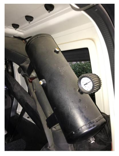
the compressor from working so hard. When used in conjunction with an air pressure shut off valve, once the reservoir tank reaches the set pressure, the compressor turns off letting it rest (even as you move from one tire to the next). Second, the reservoir allows for more efficient and constant use of air tools. It minimizes the pulsation in the system caused by a reciprocating compressor. Third, the tank allows the air to cool prior to delivery.
