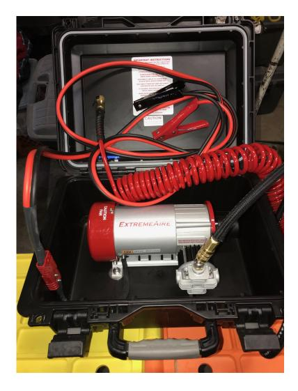
without a rest. Operation exceeding maximum pressure ratings and/or duty cycle will result in damage to the air compressor. If you decide to purchase a portable compressor for re-inflating your tires, don't forget to take it with you when leaving for an off-road trip. Also, be careful packing away vulnerable plastic hoses next to super-hot compressor heads once finished filling tires.
