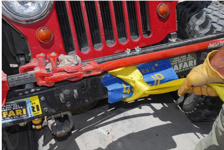
This old Willys Jeep has a very fragile front bumper, made of thin sharp sheet metal. Are you getting the story here? This is NOT a proper frame-mounted recovery point. The strap has already bent the license plate. Guess what it is going to do to the bumper once a resistance load is placed on it. Also, the "professional" trail guide looped the strap over the bumper and connected it back on itself. Very bad form. Those of you that have taken my 4WD course are cringing right now.
