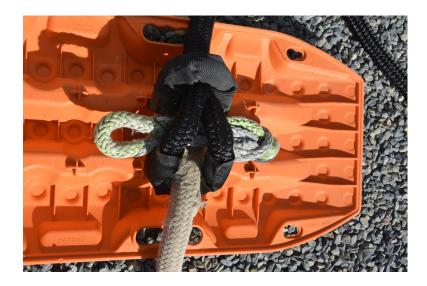
Once joined together as shown, place something light weight and flexible between the two ropes to keep them from forever being LOCKED together once pulled.
