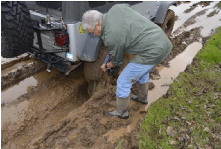
*Prior to winching, reduce the resistance of the terrain keeping your vehicle from moving. This is the easiest way to keep your winch from working so hard!*
