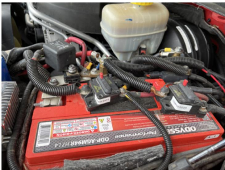
*The 6-gauge positive and negative cables routed back to my camper's battery box begin in my truck's engine compartment. The cables are connected to the positive and negative terminals on the starter battery. Visible is the 80-amp circuit breaker connected to the positive cable.*
