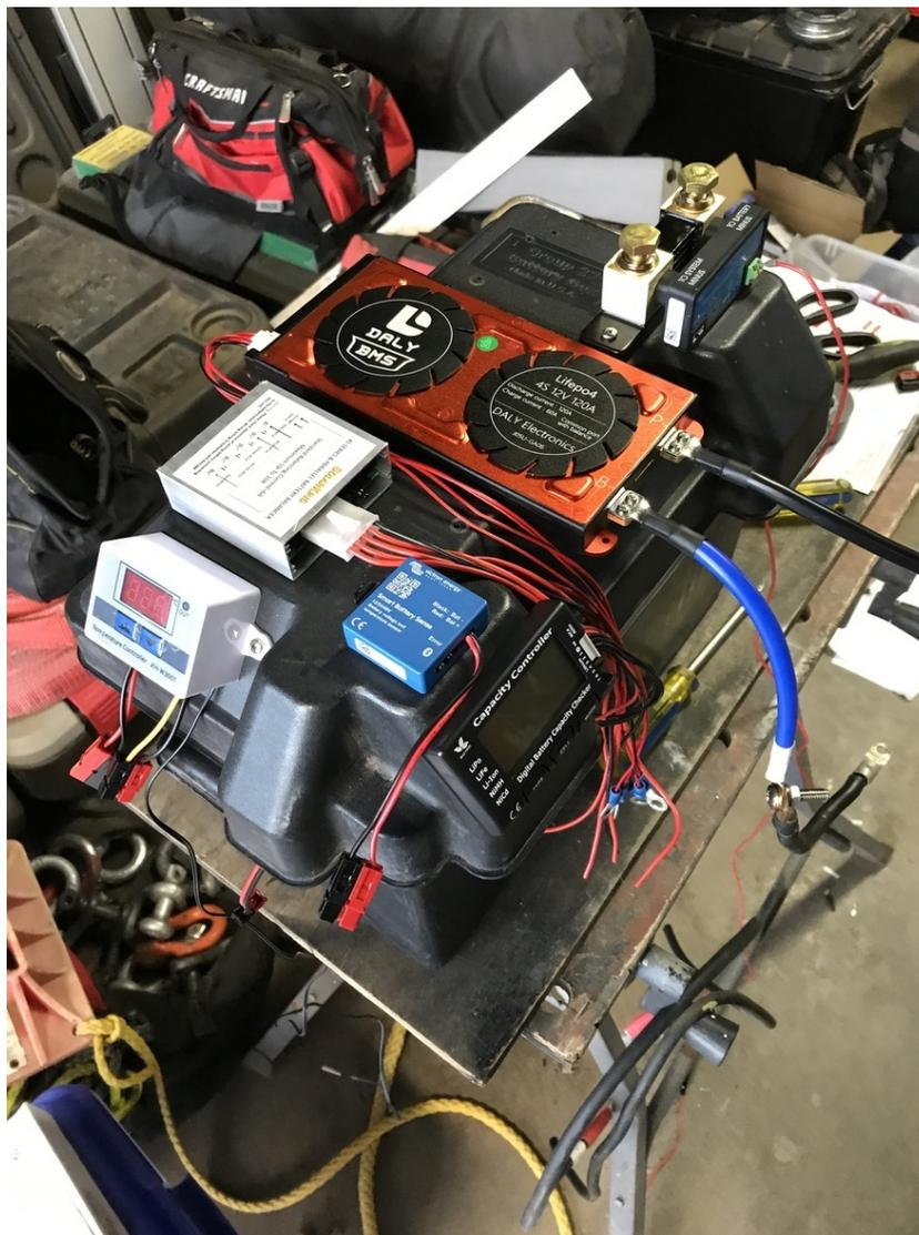
*To conduct tests on my battery box set up, I simply connected all the pieces parts and put a load on the battery prior to placing the box in my camper.*
