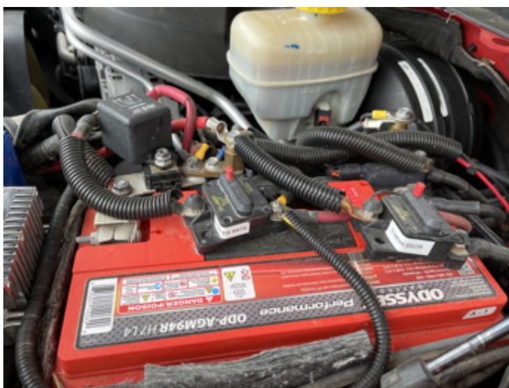
*The 6-gauge positive and negative cables routed back to my camper's battery box begin in my truck's engine compartment. The cables are connected to the positive and negative terminals on the starter battery. Visible is the 80-amp circuit breaker connected to the positive cable.*
