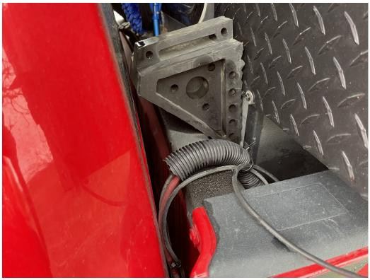
Pictured are my 6-gauge cables routed between my truck cab and bed holding my camper. The cable comes from the engine compartment, carefully routed under the cab's frame and up and over the top of the bed. The cable lays in the space between the camper and truck's bed, all the way to the camper's battery box. Obviously, I had to drill a hole into my camper's battery box to route the cable.
