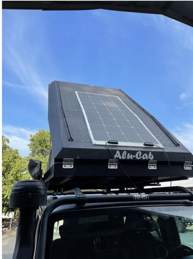
*175 Watt Renogy Flexible Solar Panel Glued on Insulation Pad and Tent Roof*
