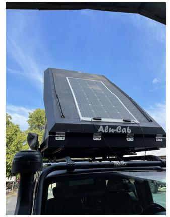
175 Watt Renogy Flexible Solar Panel Glued on Insulation Pad and Tent Roof
