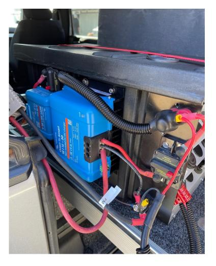
the DC/DC charger mounted on the National Luna battery box. This circuit allows the vehicle's alternator to charge the house battery while I drive.
