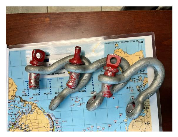
Recently there were several social media postings proclaiming that if you use a Screw Pin Anchor Shackle when rigging an off-road recovery, its pin MUST be screwed in tight. This is in contrast with the historical practice of screwing the pin all the way tight, then turning it a quarter turn backward to loosen. Let's examine both practices carefully. Some of what I'm about to write are facts and some are my personal observations.
