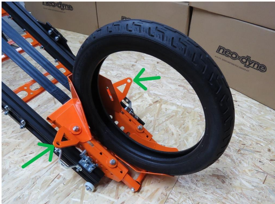
Roll the bike into the wheel chock and secure the bike to the bat wings.
