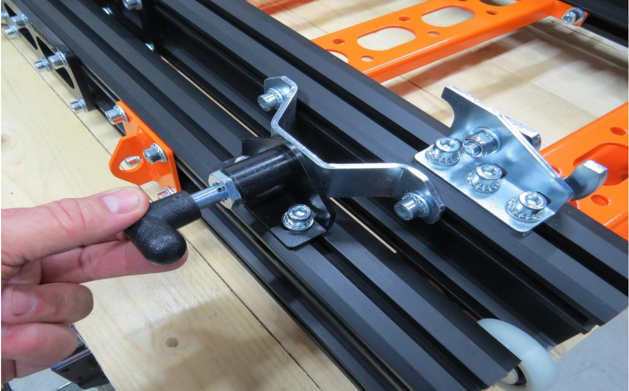
AUN210/250 : Disengage both transport locks with a gentle pull and 1/4 turn left or right.
